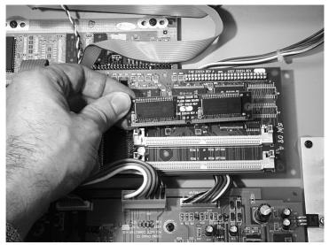
Figure 17 Proper orientation of option board
