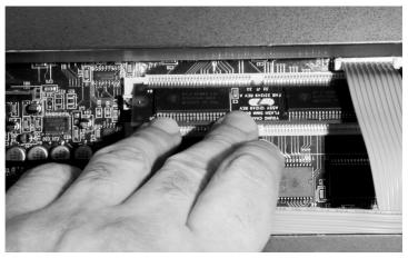
Figure 4 Placing option board in SIMM socket
