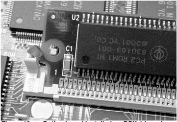
Figure 19 Option board installed on PCX-1 board
