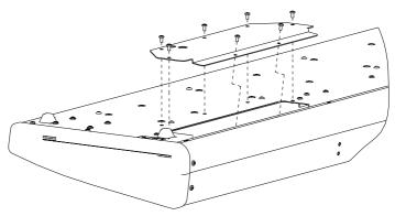
Figure 1 Removing the retaining screws
