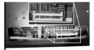
Figure 6 PCX-1 board and SIMM sockets for option boards
