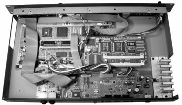
Figure 16 PCX-1 board, sockets for option boards
