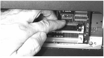
Figure 8 Placing option board in SIMM socket
