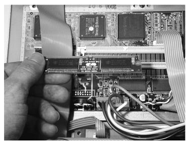
Figure 13 Proper orientation of option board
