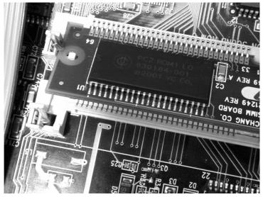
Figure 15 Option board properly installed on Engine Board
