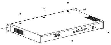
Figure 10 Removing the retaining screws
