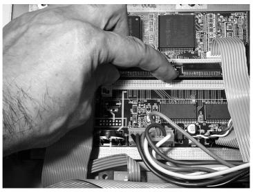
Figure 14 Placing option board in SIMM socket
