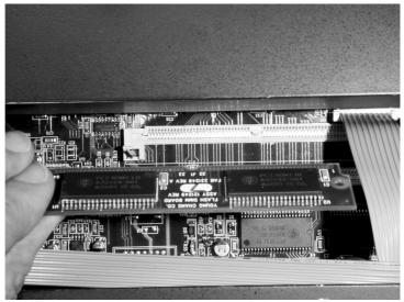
Figure 3 Proper orientation of option board
