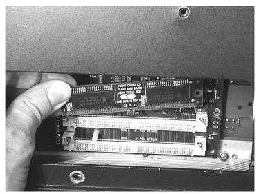
Figure 7 Proper orientation of option board
