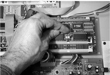
Figure 18 Placing option board in SIMM socket
