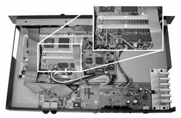
Figure 12 PC2R Engine board and SIMM sockets for option boards
