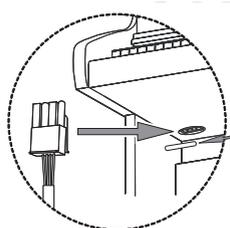
Be sure that the connector is inserted in the correct orientation.
