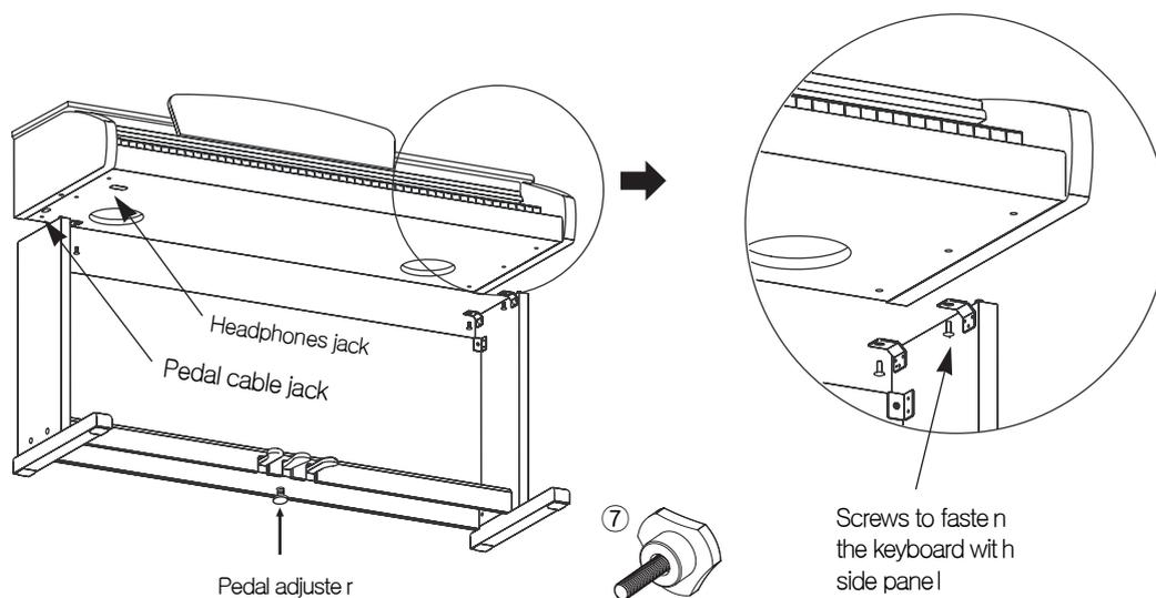
1. Place the keyboard on the stand so that the wood pegs on the bottom of the keyboard fit into the holes in the side panel brackets.
