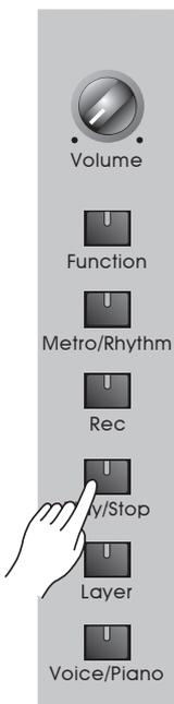
Press the [Play / Stop] button to start playback or to stop it. When the MARK PRO ONE i is in the recording mode, pressing the [Play / Stop] button will start or stop playback.
