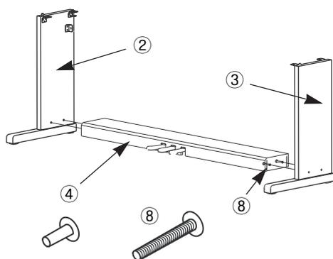
1. Place the pedal box ④ on the side panel ③ and then use ⑧ screws to fasten the side panel.
