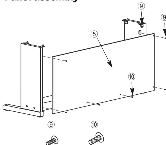
1. Fit into the holes ⑨ in the side panel brackets and then use the screws ⑨ to fasten the rear panel.
