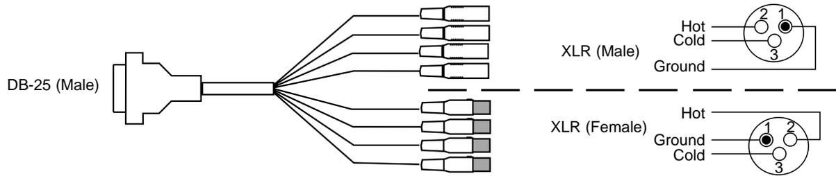
This cable allows attachment to any device that uses XLR AES connections. The DB-25 uses the pinout shown in Table 1.
