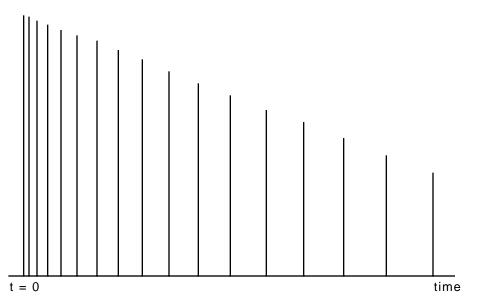
Figure 10-73 Simplified Impulse Response of LaserVerb
