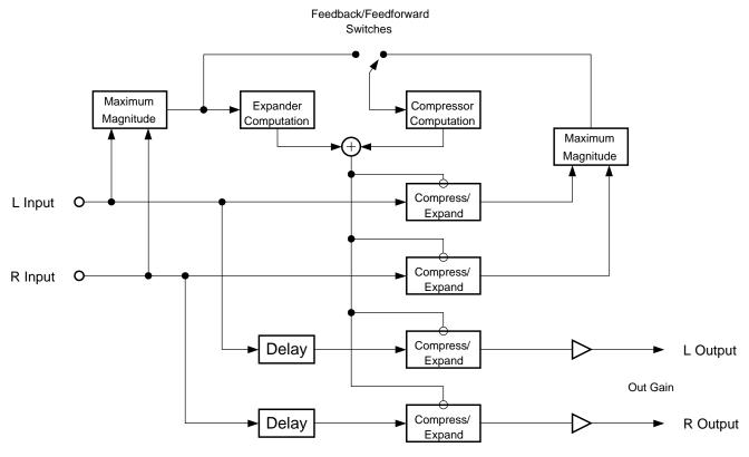
Figure 10-80 Compressor/Expander (optional EQ not shown)
