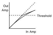
Figure 10-84 Soft-Knee Compression Characteristics
