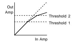
Figure 10-81 Two Segment Compression Characteristic
