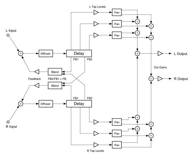
Also at the input to the delays are 1 pole (6dB/oct) lopass filters controlled by the HF Damping parameter.
