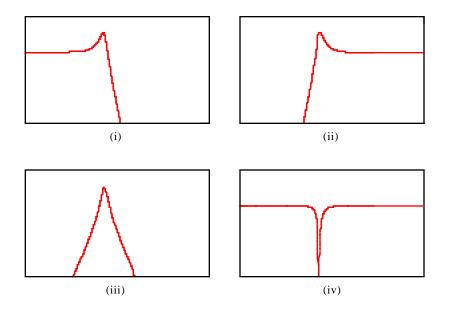
Figure 10-51 Resonant Filters: (i) lowpass; (ii) highpass; (iii) bandpass; (iv) notch
