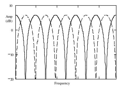
Figure 10-19 Comb Filters : Solid Line for Addition; Dashed Line for Subtraction
