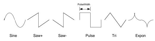
Figure 10-93 LFO Shapes available for Dual AutoPanner
