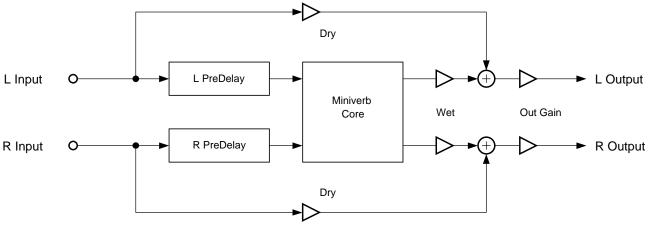
Figure 10-1 Simplified Block Diagram of MiniVerb
