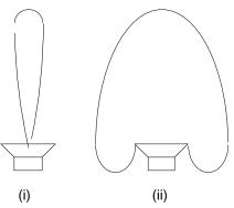
Figure 10-42 Acoustic beams for (i) low frequency driver and (ii) high frequency driver
