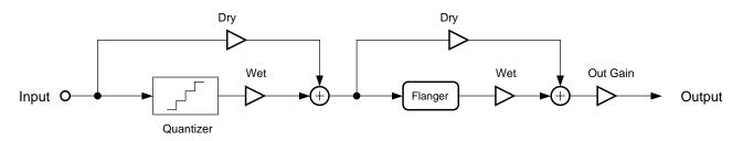
Figure 10-31 Block diagram of one channel of Quantize+Flange.
