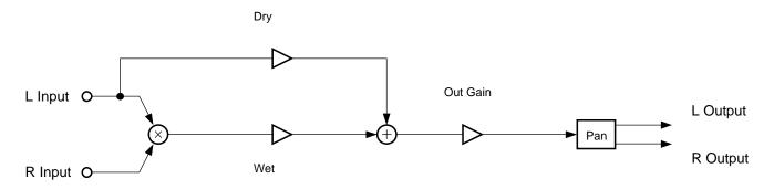
Figure 10-59 "L\*R" Mode Ring Modulator
