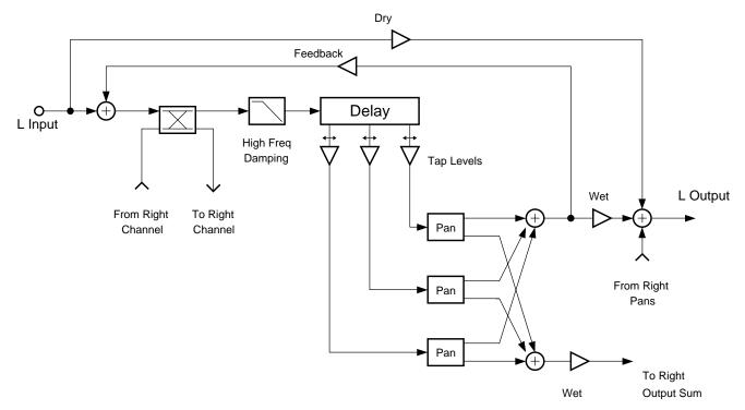
Chorus 2 is a 2 unit allocation multi-tapped delay (3 taps) based chorus effect with cross-coupling and individual output tap panning. Figure 10-11 is a simplified block diagram of the left channel of Chorus 2.
