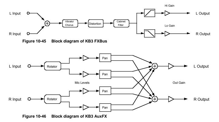
The first effect in the chain is the Hammond vibrato/chorus algorithm. The vibrato/chorus has six settings which are the same as those used in the Hammond B3®: three vibrato (V1, V2, V3) and three chorus (C1,
