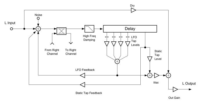
Flanger 2 is a 2 processing allocation unit (PAU) multi-sweep Thru-zero flanger effect with two LFOs per channel.
