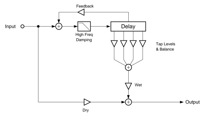
Figure 10-7 Left Channel of 4-Tap Delay
