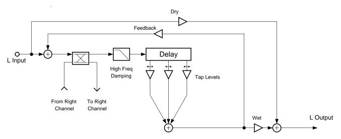
Figure 10-11 Block diagram of left channel of Chorus 2
