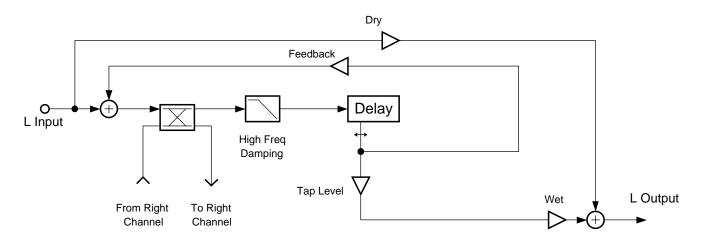
Figure 10-13 Block diagram of left channel of Chorus 1 (right channel is the same)
