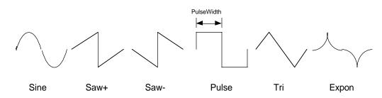
Figure 10-89 LFO Shapes available for Tremolo and Tremolo BPM
