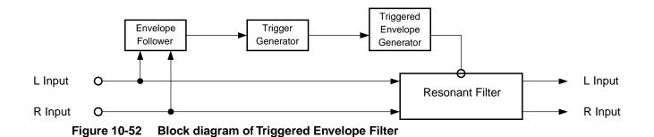
The time constant of the envelope follower may be set (Env Rate) as well as the decay rate of the generated envelope (Rel Rate). After the detected envelope rises above the Trigger level, a trigger event cannot occur again until the signal drops below the Retrigger level. In general, Retrigger should be set lower than the Trigger level. A level meter with a trigger marker is provided.
