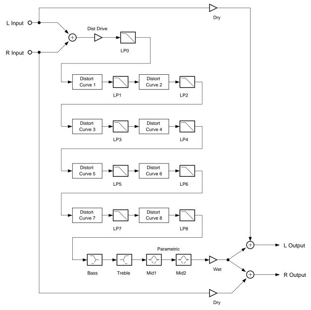
Figure 10-39 Block diagram of PolyDistort + EQ
