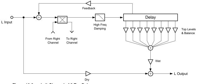
Figure 10-8 Left Channel of 8-Tap Delay
