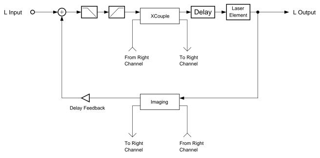
Figure 10-29 Laser Delay (left channel)
