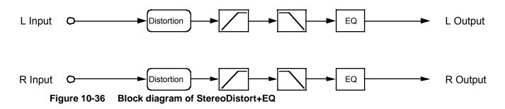
StereoDistort + EQ processes the left and right channels separately, though there is only one set of parameters for both channels. The stereo distortion has only 1 parametric mid filter.
