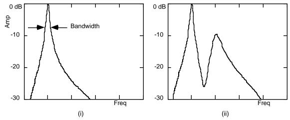
arranged in parallel and their outputs summed, so the bandpass peaks are added together and the multiple resonances are audible.
