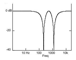
Figure 10-22 Response of LFO Phaser Twin with Wet/Dry set to 100%.
