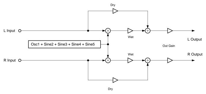
Figure 10-60 "Osc" Mode Ring Modulator
