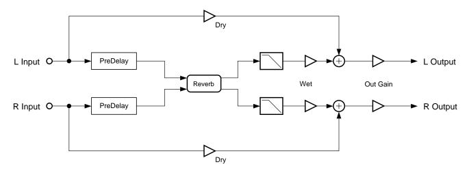
Figure 10-5 Simplified block diagram of Stereo Hall.
