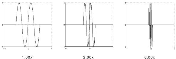
1.00x2.00xFigure 10-10Various shaper curves used in the Spectral Multi-Taps
