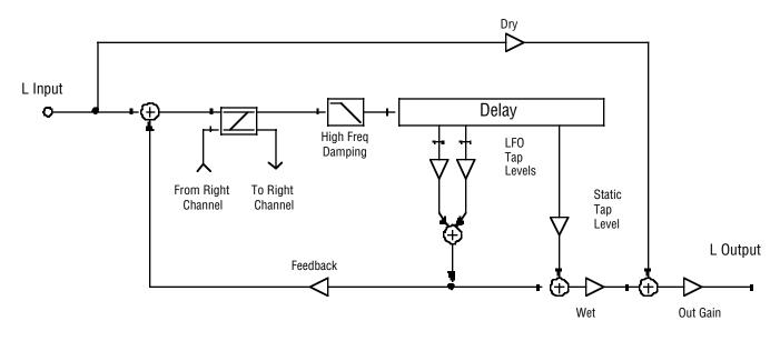
Figure 10-17 Simplified block diagram of the left channel of Flanger 1 (right channel is similar)
