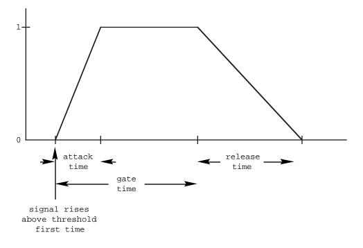
Figure 10-87 Super Gate signal envelope when Retrigger is "Off"
