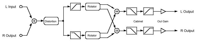
Figure 10-43 Block diagram of Distort + Rotary
