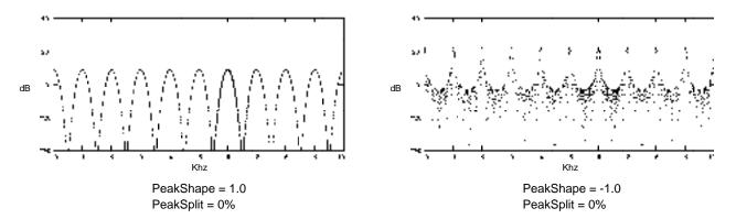
Figure 10-33 Response of Pitcher with different PkShape settings.
