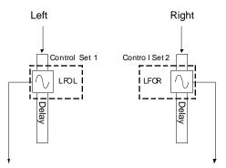
Figure 10-26 LFO control in Dual1Tap mode
