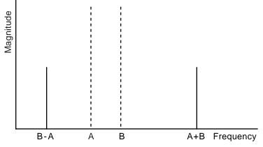
Figure 10-58 Result of Modulating Two Sine Waves A and B
