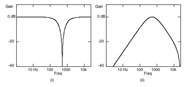
Figure 10-21 Response of typical phaser with (i) Wet/Dry = 50% and (ii) WetDry = -50%.
