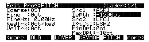
The next step is to adjust the characteristics of the stab by programming ASR1. Select the Src1 parameter again, and press **Edit** to select the ASR page.
