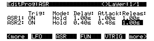
We want the stab to drop the trumpet's pitch *and* amplitude, but only when notes are played fortissimo or louder. This is done by using ASR1 as a control source on both the PITCH and AMP pages, then using a velocity trigger (VTRIG) to control ASR1.
