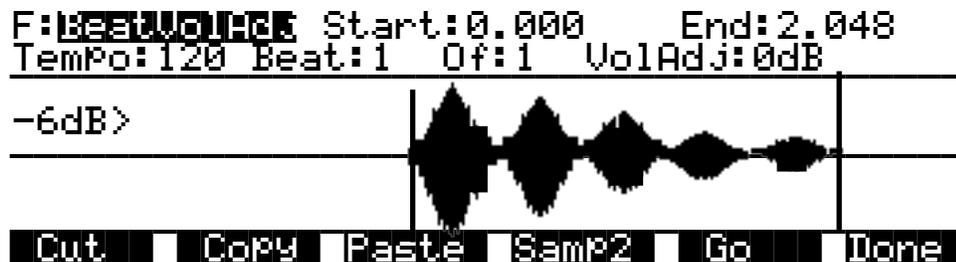
This function works much like Mix Beat. The difference is that you’re not mixing in any samples, you’re just volume adjusting Sample 1 at regular intervals. Each beat is adjusted in volume by the amount specified for the VolAdj parameter. This is useful for mixing part of a sample within itself.
