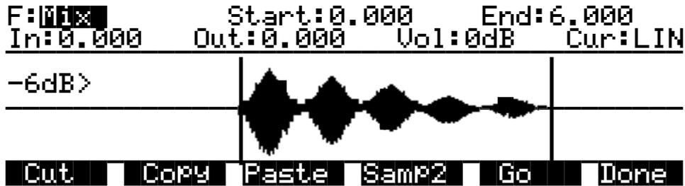
With this function you select a segment from Sample 2, and merge it with the selected segment from Sample 1, beginning at the point you set with the Start parameter. This is equivalent to mixing two audio signals through a mixing board. If the Sample 2 segment is longer than the segment from the Start (S) to the End (E) of Sample 1, the resulting sample will be longer than the original Sample 1.
