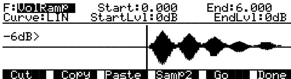
This function lets you apply a ramp to the volume of the selected sample range. The Start Level and End Level parameters let you set the amount of cut (negative value) or boost (positive value) at the start and end points of the segment. The Curve parameter determines the shape of the ramp that scales the amplitude of the sample between the start and end amplitudes. The available values are LIN, EXP, COS, EQL, and MIX. These curves are described at the end of the section on DSP functions.
