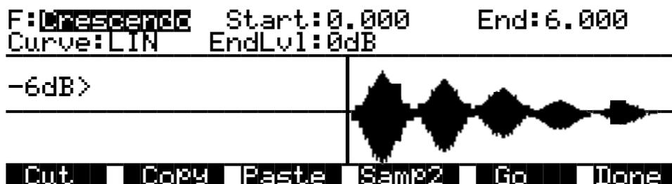
Similar to Volume Ramp, this function applies a curve that scales the amplitude of the selected sample segment. Unlike Volume Ramp, however, you simply select a start and end point, and a single level. The amount of cut or boost starts at 0dB at the start point of the ramp, and reaches the level you specify when it reaches the end point of the ramp. The samples after the end point are scaled to the amplitude level of the end point.
