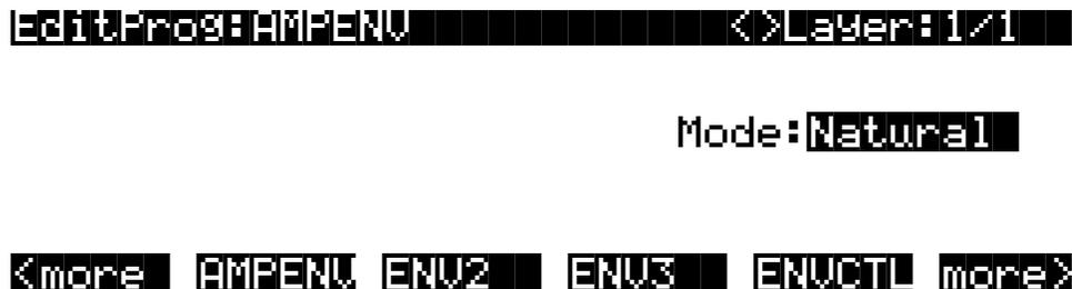
If you want to build your own amplitude envelope, just turn the Alpha Wheel a click. The word "Natural" will change to "User," and a set of AMPENV parameters will appear. The sound will change when you do this, because the default settings for the User envelope, as shown in the diagram below, take effect as soon as you leave Natural mode. Returning to Natural mode applies the original amplitude envelope once again.
