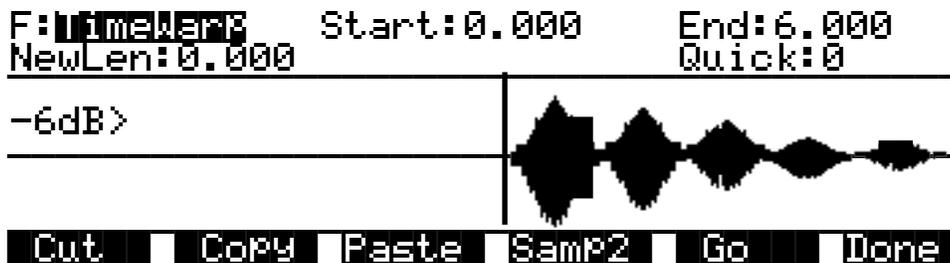
With this function you can change the length of the selected sample segment without affecting the pitch. This function applies sophisticated routines that lengthen or shorten the selected sample segment to play it back over an different time period, modifying the playback rate so the pitch remains unchanged.
