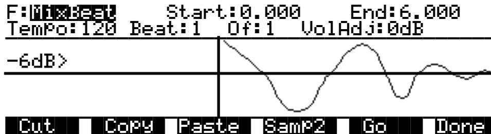
With this function you can mix the selected range of Sample 2 into Sample 1 at regular intervals. The most natural application of this function is to add percussion samples, but it can be used to mix any sample at regular programmable intervals (beats).
