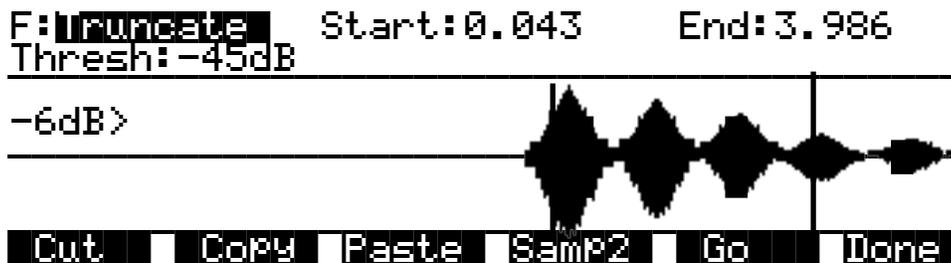
The Truncate function will automatically reset the Start (S) and End (E) points of the sample. This can be quicker than trimming the sample manually on the TRIM page.
