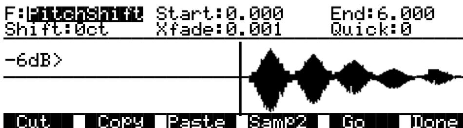
The PitchShift function is the counterpart of the TimeWarp function; it shifts the pitch of the selected sample segment without changing the playback time—very useful for tuning samples when the playback time is crucial. Use the Start and End parameters to define the segment to be shifted. The Shift parameter determines the amount of pitch shifting, up to  $\pm 30000$  cents.
