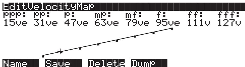
The top line of the display gives you the usual reminder of your location. The bottom line labels the soft buttons, which execute the normal librarian functions of naming, saving, or deleting velocity maps, or dumping them via SysEx. The values you see in this diagram are the settings for the velocity map 1 Linear.
