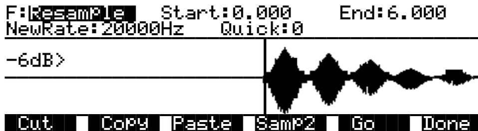
Use this function to change the sample rate of the samples in the selected segment. This is convenient for converting samples to new rates matching those of other samples to be mixed with or inserted into. It's also useful for saving memory and altering the timbre of a sample.
