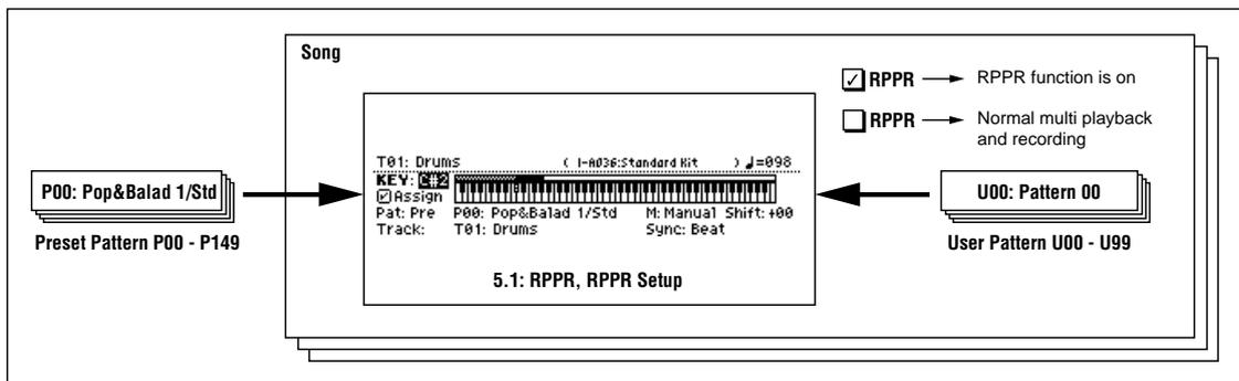
You can make assignments for keys C#2–C8. Keys C2 and below are used for stopping the pattern playback, and cannot be assigned.
