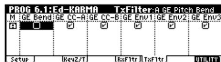
Here you can specify whether to apply filtering to the MIDI control data transmitted by the KARMA module. If an item is **On (checked)**, it can be transmitted.
