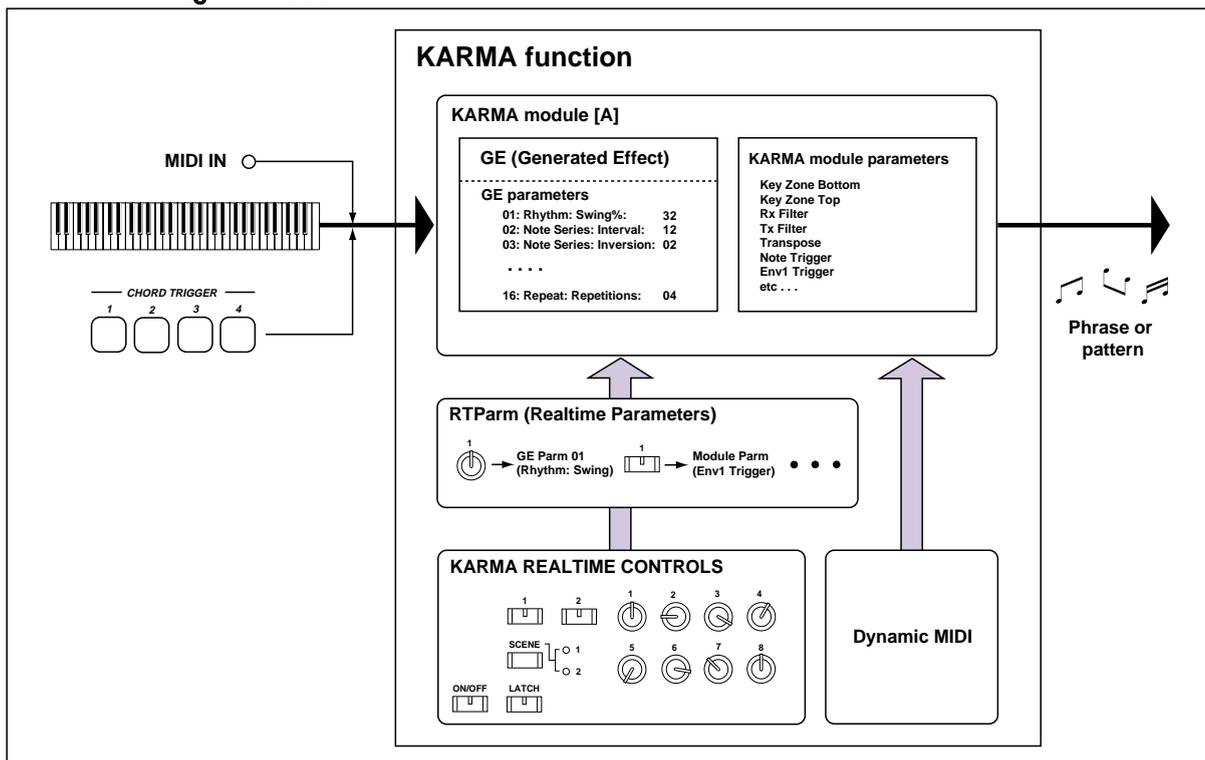
GE parameters and KARMA module parameters can be assigned to the KARMA Realtime Controls knobs and switches, allowing you to control these phrases in realtime while you play, so that you can freely modify the phrases or patterns.
