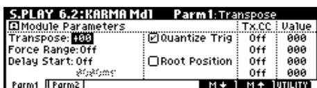
The trigger timing will be quantized to the nearest 16th note interval of the SMF beat.
