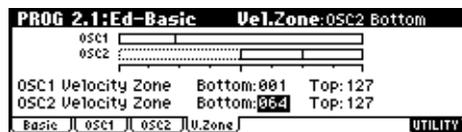
Here you can specify the range of velocities that will sound oscillators 1 and 2. In the example shown above, the velocity ranges are as follows.
