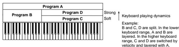
As an additional possibility, you can set the slope for a key zone or velocity zone so that the volume diminishes gradually. This lets you change a split into a **keyboard crossfade**, or a velocity switch into a **velocity crossfade**.
