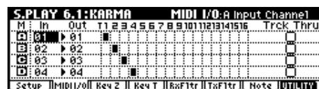
Set the KARMA module [A] "Input Channel" and "Output Channel" to 01 and 01 respectively. Set the KARMA module [B] "Input Channel" and "Output Channel" to 02 and 02 respectively.
