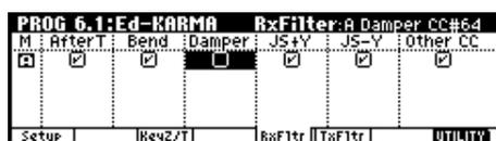
Here you can specify whether filters will be applied to the MIDI control data received by the KARMA module before it is passed on (echoed) to the tone generator.
