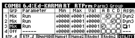
In the same way as for a program, set "Grp," "Parameter," "Min," "Max," "Val," and "Asgn." In a combination, you can use KARMA modules [A], [B], [C], and [D]. Turn "Param Module" On (checked) for the modules that you wish to control. In the example shown above, KARMA Realtime Controls switch [1] is controlling Run/Mute for modules [A] and [B], and switch [2] is controlling Run/Mute for modules [C] and [D].
