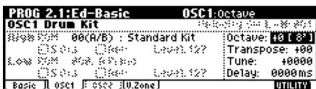
In the Basic (Prog Basic) page, set “Mode (Oscillator Mode)” to **Drums**. When this is set to **Drums**, you will be able to create a drum program. This will select a **drum kit** instead of a multisample. This instrument provides sixteen factory preset drum kits that are suitable for a wide variety of music. (≡Drumkit name, VNL) Here you can only select a drum kit. To edit or create a drum kit, use GLOBAL 5.1: DKit (≡p.90).
