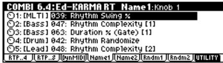
In a combination, part of the category name of the program selected for the timbre controlled by the KARMA Realtime Controls knobs and switches is automatically displayed in square brackets [ ]. If settings have been made to control multiple timbres simultaneously, this will indicate [MLTI].
