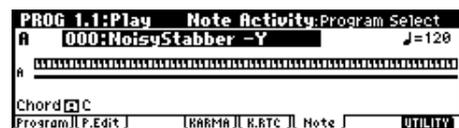
When you play the keyboard or press a CHORD TRIGGER [1]–[4] key, “Chord[A]” will indicate the name of the chord detected by the KARMA module. “Note Activity Display” will display the notes generated by the KARMA module.
