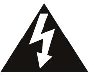
CE SYMBOLE A POUR BUT D'AVERTIR L'UTILISATEUR DE LA PRÉSENCE DE VOLTAGE DANGEREUX NON-ISOLE A L'INTÉRIEUR DE CE PRODUIT QUI PEUT ÊTRE DE PUISSANCE SUFFISAMMENT IMPORTANTE POUR PROVOQUER UN CHOC ELECTRIQUE AUX PERSONNES.
