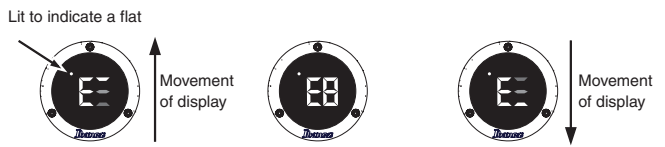
When the pitch is low When the pitch is correct: E-flat When the pitch is high
