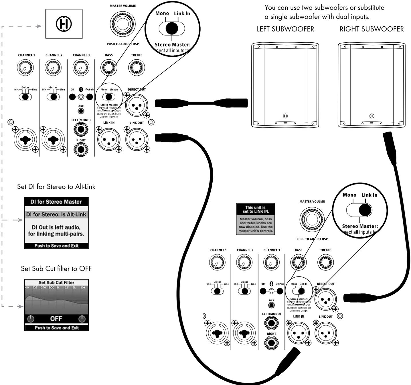
You can use two subwoofers or substitute a single subwoofer with dual inputs.
