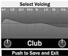
Turn the Master Volume/DSP knob to set the displayed function. On this page, the Master Volume/DSP knob selects the Voicing.
