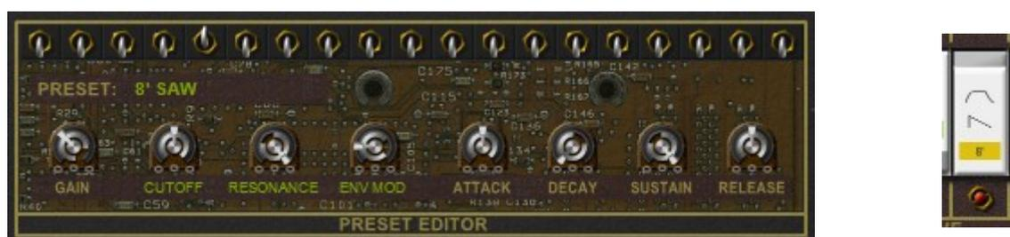
What you see are the eight (in case of "16' PWM" nine) parameters that affect the character of a preset. To select the "right" editor for a preset you can either flip one of the switches above the Preset Editor, activate the preset via its Rocker switch, or push one of the red kick switches that appeared right under the Rocker switches once you "opened" the Preset Editor.
