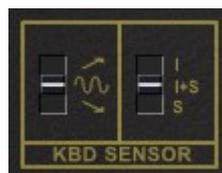
While the intensity of the effect is controlled in the *Effects* section (see above), the destination can be set to *Pitch Bend Up*, *Pitch Bend Down*, or *Vibrato*. Furthermore, one can activate it for the *Instrument* or the *Synthe* section alone or together.
