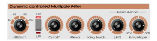
The dynamic filter is a traditional multi-pole VCF architecture with several modulation options and variable key-tracking. In addition the filter has an overdrive-stage on the output, before going in to the 7-band static filter.
