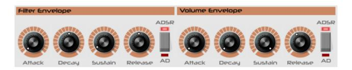
The filter envelope generator and volume envelope generator are identical and hard-wired to their respective destinations. The envelope generators are of the traditional ADSR-type, meaning Attack, Decay, Sustain and Release. They can be switched from ADSR to AD mode for percussive sounds.
