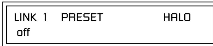
4. Move the cursor to the second line of the display. Select the preset you want to link with the preset you selected in step 1. Play the keyboard as you scroll through the various presets to hear the results.
