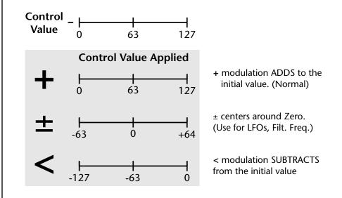
"+" Modulation: Uses only the positive half of the range, adding to the current value. For example, if the filter frequency were set to 100 and you patched Vel+ to the filter, the filter frequency would increase from 100 as velocity was applied.
