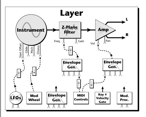
• Note-on modulation sources, such as key, velocity and gate output a single value at note-on time. Realtime modulation sources such as LFOs, envelope generators and modulation wheels output continuously changing values.
