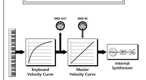
The Keyboard Velocity Curve modifies the velocity data from the keyboard keys. This data is sent to the MIDI output port and through the Master Velocity Curve before reaching the Synthesizer. Incoming MIDI data is filtered through the Master Velocity Curve only.
