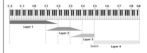
With a High Fade value of zero (as in layer 3 of the diagram), the layer simply switches off at the high key.
