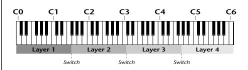
Just assign the low and high key range for each of the four layers with Fade set to zero. Set the Low and High Keys so they don't overlap other layers.
