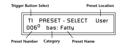
When a preset is selected using the Preset Select buttons, the cursor is automatically located underneath the Preset Name field. This feature makes it easy to select other presets of the same type.
