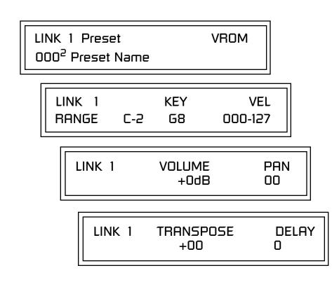
Links provide an easy way to create new sounds by combining the existing presets. Or, you can create your own custom stacked presets with up to 12 layers! We're talking LARGE sounds here. Of course Links can also be used when you just want to stack up two sounds.
