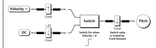
Connect the DC level to the input of the switch along with the velocity value. Note that more than one modulation source can be applied to the input of a processor.
