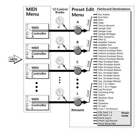
External MIDI controller numbers are assigned to the Letters A-P in the MIDI menu. The Initial Controller Amount value is sent to the PatchCord destination when the Preset is first selected. If you move the Control Knob, then that value replaces the initial value. If MIDI controller data is received it will similarly replace the knob or initial setting.
