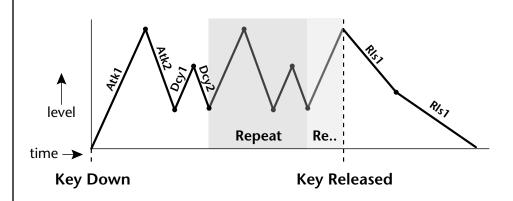
The diagram above show how the looping envelopes work. When the key is pressed the envelope goes through its regular Attack 1, Attack 2, Decay 1 and Decay 2 stages. In non-looping mode, the envelope would hold at the end of the Decay 2 stage until the key was released. In looping mode however, it jumps back to the Attack 1 stage and repeats the first four stages. It continues to loop through these four stages until the key is released where it immediately jumps to the Release 1 stage.
