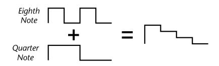
Adding these two clocks together in equal amounts produces a stairstep waveform.
