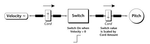
The patch illustrated above is programmed by setting the PatchCord screens as shown below.
