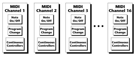
Any MIDI controller can be routed to any modulation destination. First, you have to know which controller numbers your keyboard transmits. Most modern MIDI keyboards let you select a controller number for each control on the keyboard. For example, it may let you select a number from 0-31 for the data slider. The realtime controller numbers that the keyboard transmits must match the numbers Vintage Keys is receiving, otherwise nothing will happen when you move the controls.
