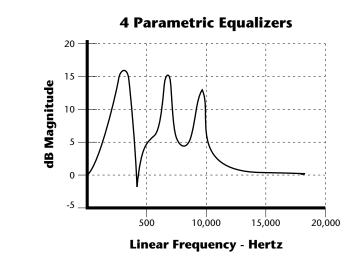
Many natural instruments have complex resonances which are based on their soundboard or tube size. The resonance shown above would be impossible to create using a normal synthesizer filter.
