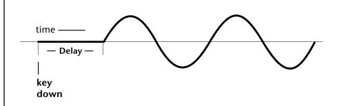
All Delay values equal to or greater than zero specify absolute time rates from 0 to 127. Values less than zero specify Tempo-based mode. Refer to the previous table for times and tempo-based rates.
