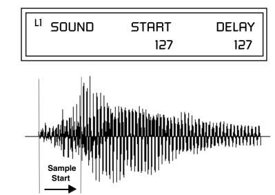
Controlling the Sound Start using Key Velocity (< Amt -) brings in the attack of the wave only when you play hard. This is especially effective with percussion instruments.
