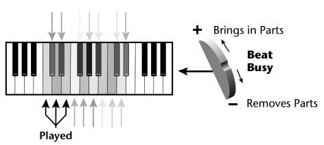
Positive controller values bring in new Parts and negative controller values remove Parts that are latched or held. In this example, the Pitch Wheel is connected to Beat Busy since it outputs negative as well as positive values.
