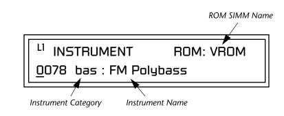
To select an instrument for the selected layer(s), move the cursor to the bottom line of the display and change the instrument using the data entry control.
