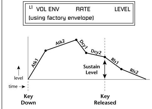
On the Volume Envelope, levels can only be set to positive values. The value range is from 0 to +100.
