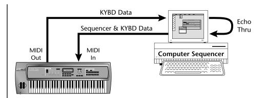
Turning Local Control Off allows you to use the Echo Thru feature on your sequencer while sequencing. In conjunction with Echo Thru, Local Control Off allows you to record into the external sequencer and hear the correct sounds whether you are recording or playing back the sequence.
