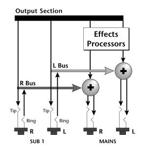
You can use the Sub 1 jacks as effect returns to the Main Outputs. Note that the Effects Processors are only routed to the Main Outputs.
