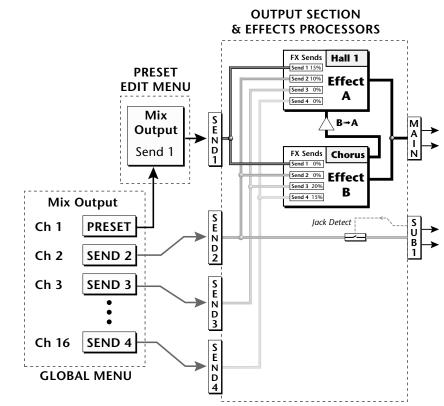
Individual layers or entire MIDI channels can be routed to any of the four busses.
