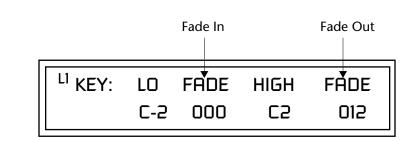
Layers can be crossfaded according to key position by adjusting the Low and High Fade parameters. The first Fade field determines how many semitones it takes the layer to Fade In from the low key. The second Fade field determines how many semitones it takes the layer to Fade Out to the high key. The screen shot above and the diagram below show Layer 1 being faded out over a one octave range.
