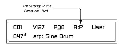
All arpeggiators share Vintage Keys's master clock and its current setting. The master clock can be Vintage Keys's internal clock or an external MIDI clock (page 82). Although the arpeggiators use the master clock setting, the tempo divisor can be unique for each arpeggiator setup.
