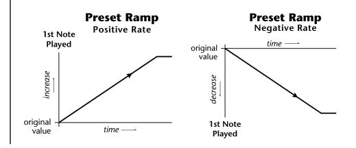
The preset ramp instantly resets when all notes have been released and the next *first key* on the MIDI channel is pressed. The Ramp Rate polarity (+ *or* -) determines if the ramp will be positive or negative going. The value of the ramp rate sets the increment. Large values produce fast ramps and small values produce slow ramps. Multiple inputs can be connected to the ramp rate (just like all the other destinations in Vintage Keys).
