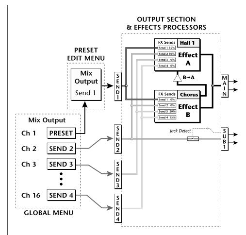
The Mix Output screen in the **Global** menu assigns each MIDI channel to a Send (1-4) or to "Preset".
