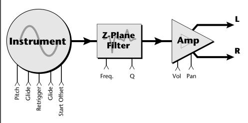
To understand how a filter works, we need to understand what makes up a sound wave. A sine wave is the simplest form of sound wave. Any waveform, except a sine wave, can be analyzed as a mix of sine waves at specific frequencies and amplitudes.
