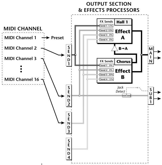
Send 2 can be routed to the effects processors or to rear panel submix jacks. When a plug is inserted into a Submix jack, the dry portion of the Send is disconnected from the effects processor and is routed **directly** to the Submix output jacks.
