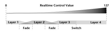
After the Ranges and Fades have been adjusted for each layer in the Realtime Crossfade screen, you must assign a real-time controller to RTXfade (Real-time Crossfade) **on each Layer** in the PatchCord screen. Set the PatchCord Amounts to +100.
