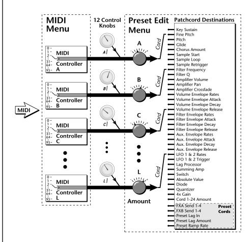
MIDI A-P are internal connections which simultaneously carry front panel controller knob data and MIDI continuous controller data.
