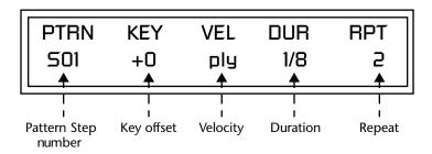
**3.** Move the cursor to the **lower line** of the display. For each step, you can select: key, velocity, duration, and number of repeats.
