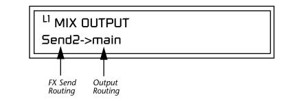
The Sends function as effect processor inputs (effect sends). The Output Routing field shows the true routing of the Sends to the Main output.
