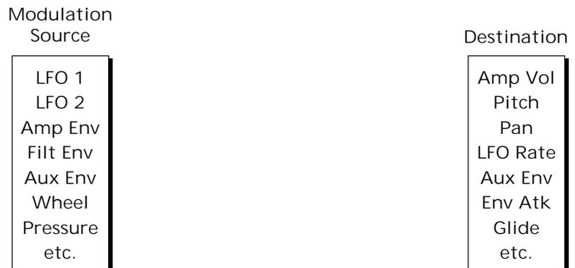
Each patch has an amount field which determines how much modulation is applied to the destination. The modulation amount can be positive or negative. Negative values invert the input. The amount value range is from -100 to +100.
