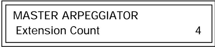
For example, with the Extension Interval set to 12 (an octave) and an Extension Count of 2, and with the Arpeggiator Mode set to Fwd Assign, if you played E2, then C2, then G2, the arpeggiated sequence would consist of: E2, C2, G2, then E3, C3, G3, and then E4, C4, G4. The Extension Count values range from 0 through 15. Refer to the following illustration.
