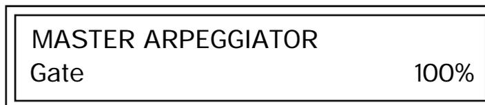
With a Gate Time setting of 100% the note is held on until the next note starts. The envelope generators never advance to the Release stages. With a Gate Time setting of 50%, the note is released halfway through the note cycle and the envelope generators proceed to their release stages until the next note occurs. Refer to the following illustration.
