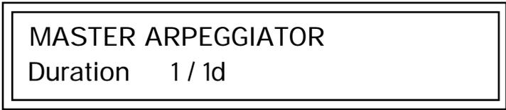
Duration can be used to modify the patterns and increase the possible pattern combinations and variations. Because this parameter limits the length of arpeggiator play time, it can change the arpeggio pattern when the Duration is less than the length of the arpeggio. You can set the arpeggio to repeat continuously using the *Recycle* function described below.
