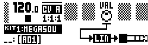
**VAL** (Value) sets the voltage level of the CV. Applicable when the chosen CV type is VALUE LIN.
