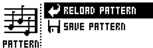
**RELOAD PATTERN** will reload the active pattern. It will either be reloaded to its original auto-saved state or to a specific saved state which can be determined by utilizing the **SAVE PATTERN** command. Press **[NO/RELOAD] + [PATTERN]** for a short cut to the **RELOAD PATTERN** command.
