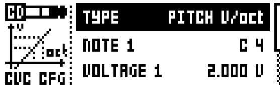
Please read the following paragraphs on how to set up CV pitch control. CV pitch is configured by finding the voltages generating two different notes from the synthesizer you wish to control. To get a good result you should select the notes two or three octaves apart.
