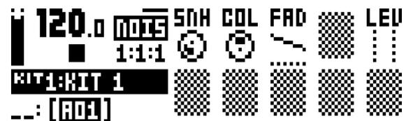
**S&H** (Sample & Hold) sets the tuning of the noise spectrum.
