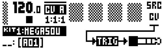
**SRC** (Source Track) sets the track to use for sending trig signals. The CV track, FX track and synth tracks 1-4 can be used as source.
