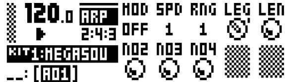
**MOD** activates the arpeggiator and controls how the arpeggiated notes will be cycled.
