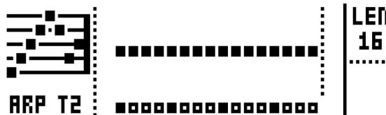
Select the length of the arpeggio by turning **DATA ENTRY** knob **E**. The max length is 16 sequencer steps. The <TRIG LEDS> indicate the length of the arpeggio and, when the arpeggio is playing, the number of played arpeggio notes.
