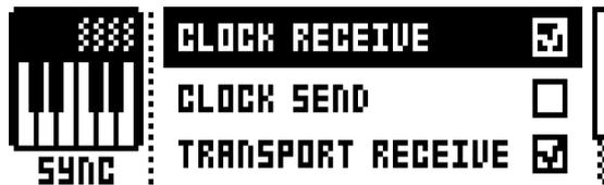
**CLOCK RECEIVE** will when active make Analog Keys respond to MIDI clock sent from external devices.
