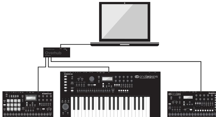
The Overbridge software suite enables a tight integration between the Analog instruments (Analog Rytm, Analog Keys, Analog Four) and a computer DAW.
