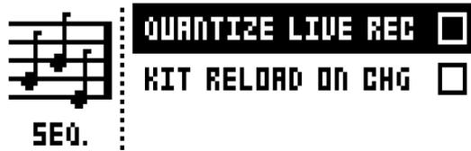
**QUANTIZE LIVE REC** will when active quantize notes entered in LIVE RECORDING mode to complete sequencer steps. When the setting is deactivated, live recorded notes will where applicable be affected by micro timing. Read more about micro timing in the section "NOTE MENU" on page 37.
