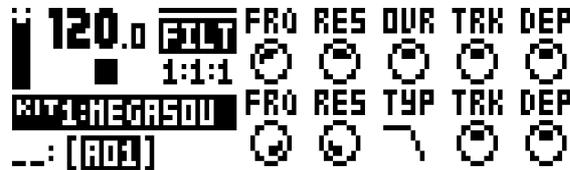
6. Place note trigs on the first step of the sequencer. It is necessary to trig the amplitude envelope.
