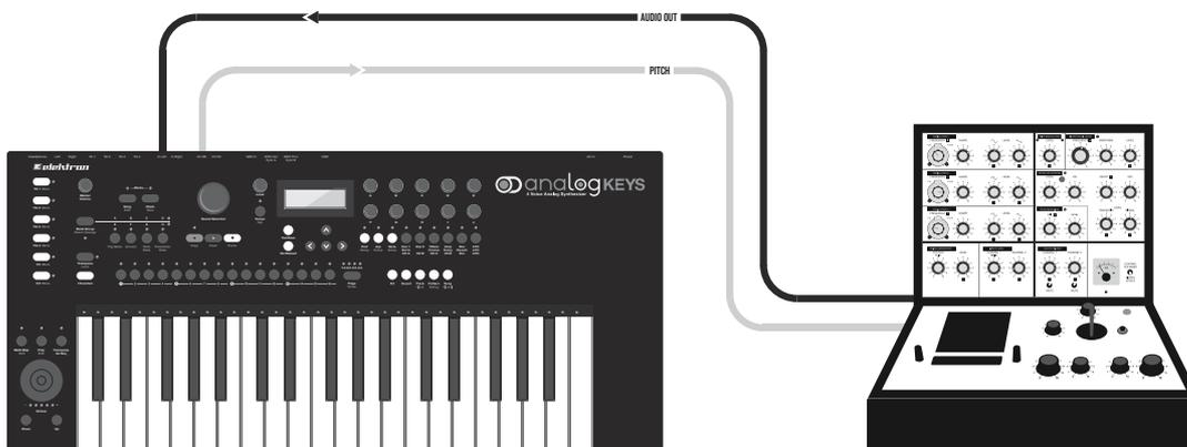
The CV/Gate outputs and the external inputs allow an external oscillator to be used with the internal Analog Keys oscillators. Use this trick when you want a different (perhaps old, quirky and unpredictable yet charming) oscillator to provide the fundamental tone but still want the control and modulation power of Analog Keys.
