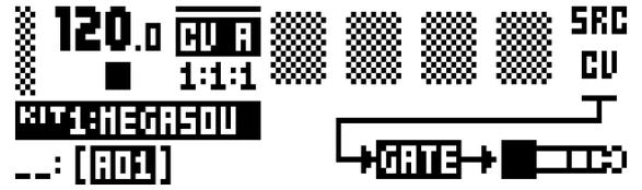
**SRC** (Source Track) sets the track to use for sending gate signals. The CV track, FX track and synth tracks 1-4 can be used as source.
