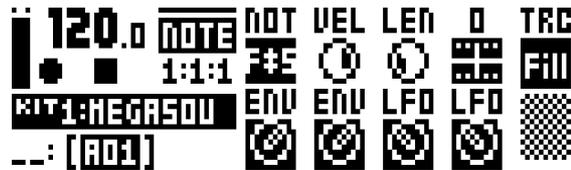
The sequencer needs to be in fill mode in order to activate the parameter locks called FILL (see below). Fill mode is activated, for one pattern cycle, by pressing [YES] + [PAGE]. It will become active when the pattern loops, and remain active until it loops again.
