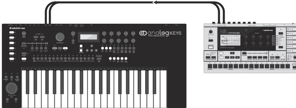
Thanks to the neighbor routing, all the filters of Analog Keys can be used for providing an immense mono filter-bank consisting of 8 filters plus 4 overdrive circuits. The setup can be either serial or parallel. It can of course be set up for stereo filtering as well. In this scenario 4 filters are available for the left and right channels.
