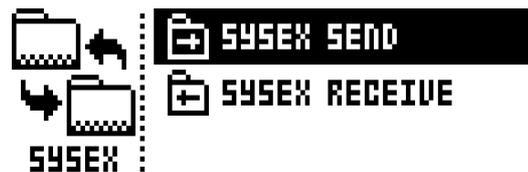
When receiving or sending SysEx data, the MIDI ports or the USB port of Analog Keys must be connected to the external sending/receiving device.
