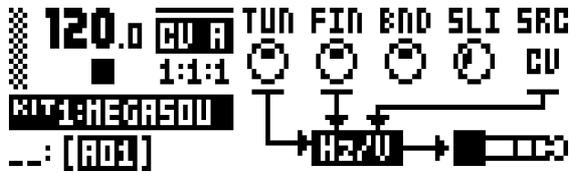
**TUN** (Coarse Tune) sets the coarse tuning of the CV in semi-tones.
