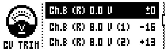
Each CV output has three trim settings. Begin by selecting 0 V, then press and hold the **[YES/SAVE]** key. 0 V is output as long as **[YES/SAVE]** is held down. Use **[ARROW]** keys **[LEFT]** / **[RIGHT]** or **DATA ENTRY** knob **A** to adjust the voltage until your voltmeter shows exactly 0 V. Repeat the process for both 8 V settings (the first one is for continuous voltage, the second is for pulse).
