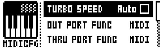
**TURBO SPEED** selects the multiplier of the MIDI transfer rate that will be used when Analog Keys MIDI IN/OUT ports are connected to the MIDI OUT/IN ports of a turbo protocol compatible device. The [LEFT]/[RIGHT] arrow keys are used to select the multiplier. If AUTO is chosen, press [YES/SAVE] to start the turbo speed negotiation.
