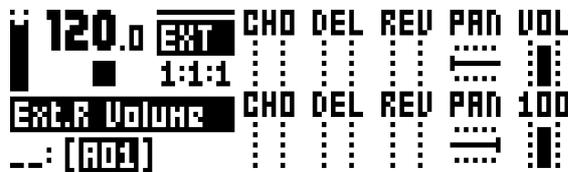
3. Make a performance macro controlling the CHO, DEL and REV parameters, located on the EXT IN page of the FX track, for both the left and right channel. See page 20 on how to make a performance macro.
