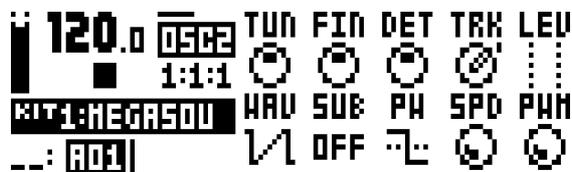
**TUN** (OSC2 Coarse Tune) sets the pitch of the oscillator in semitones. To jump a whole octave, press the knob while turning it.
