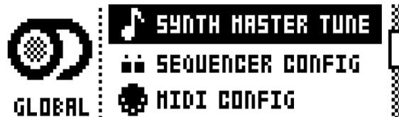
**SYNTH MASTER TUNE** Sets the master tune for the analog oscillators. The default setting is the international standard middle A, 440.0 Hz. The tuning across all octaves is done according to the 12-TET convention.
