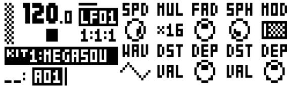
**SPD** (LFO1 Speed) sets the speed of LFO1. It is synced to the BPM. For LFO1 to be synced to straight beats, try settings of 16, 32 or 64. The value is bi-polar (the LFO shape can be played backwards by using negative values).
