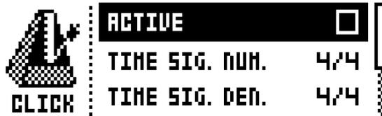
**ACTIVE** activates/deactivates the metronome. It is also possible, outside of this menu, to keep **[FUNCTION] + [TRACK]** pressed for a second to toggle the metronome click on or off.
