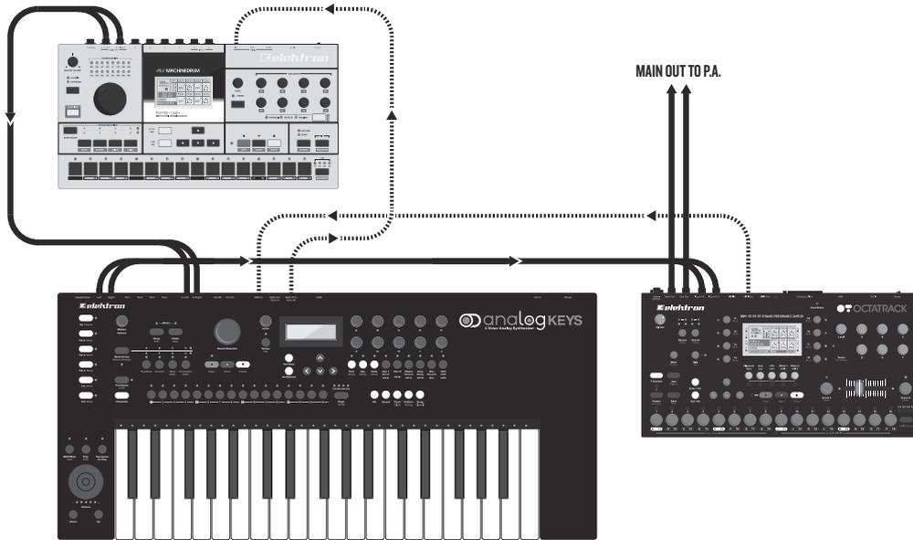
Analog Keys really thrives with other Elektron gear. In this example it is used with an Octatrack and a Machinedrum. The Machinedrum main output is connected to Analog Keys inputs. Analog Keys main output is connected to one of the input pairs of the Octatrack. The main outputs of the Octatrack goes to the PA. The Machinedrum and Analog Keys are MIDI slaved to the Octatrack.
