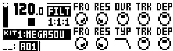
**FRQ** (Filter1 Frequency) sets the cutoff frequency of Filter 1, the 4-pole lowpass transistor ladder filter.
