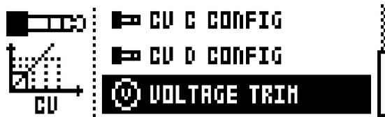
Make sure you have a good voltmeter before proceeding. Connect a TRS cable to the output you want to trim. Connect the volt meter's negative terminal to the sleeve of the connector. Connect the positive terminal to either the tip or the ring of the connector, depending on the channel you wish to trim.
