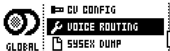
Activate/deactivate routing of any the four voices to the main output and to the FX track. Navigate using the **[ARROW]** keys. Tick or untick box with the **[YES/SAVE]** key.
