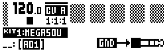
No parameters available. The CV output will not send any signal.
