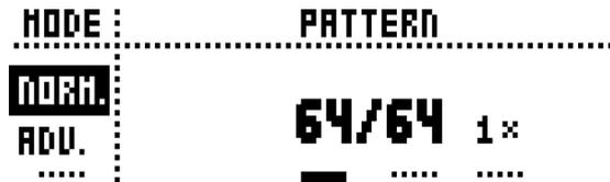
The first two settings control the step length of the pattern. The leftmost number selects the number of steps in the pattern. The maximum number of steps available to the pattern is determined by the total length, set by the parameter to the right. This can be either 16, 32, 48 or 64 steps. If 17 steps or more are used in a pattern, the **[PAGE]** key is, while in GRID RECORDING mode, used to toggle between the different pattern pages.
