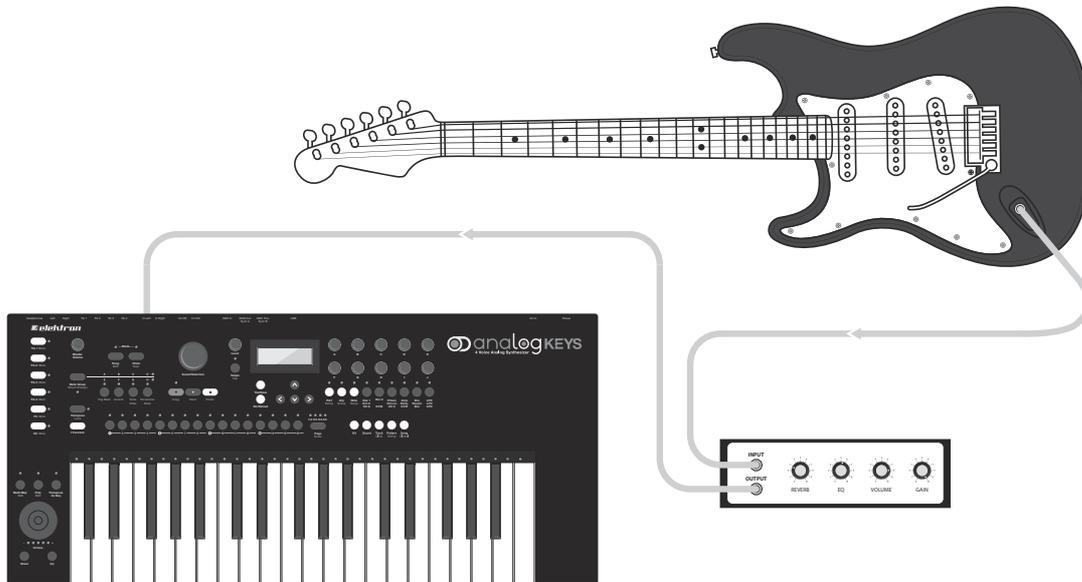
In this setup example Analog Keys is used for processing the sound output from an electric guitar. The first, most basic method uses the FX track to turn Analog Keys into an effects box sporting the Wideshift Chorus, Saturator Delay and Supervoid Reverb effects. The second, more elaborate method routes the sound through Track 1 and allows all the sound-shaping possibilities offered by the FILTERS, AMP, ENV and LFO.
