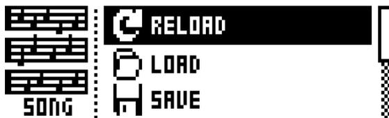
**RELOAD** will reload the active song. It will be restored to its saved version. Press **[NO/RELOAD] + [SONG]** for a short cut to this command.
