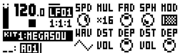
**SPD** (LFO1 Speed) sets the speed of LFO1. It is synced to the BPM. For LFO1 to be synced to straight beats, try settings of 16, 32 or 64. The value is bi-polar, meaning the LFO shape can be played backwards by using negative values.
