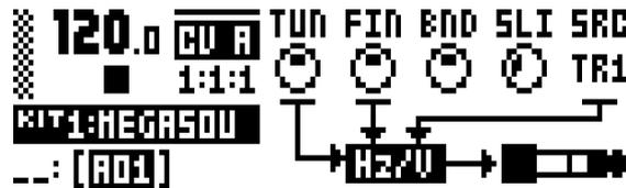
6. Select track 1. Set **WAV** on the OSC1 page to IN L. For oscillator 2, choose one of the internal Analog Keys waveforms.
