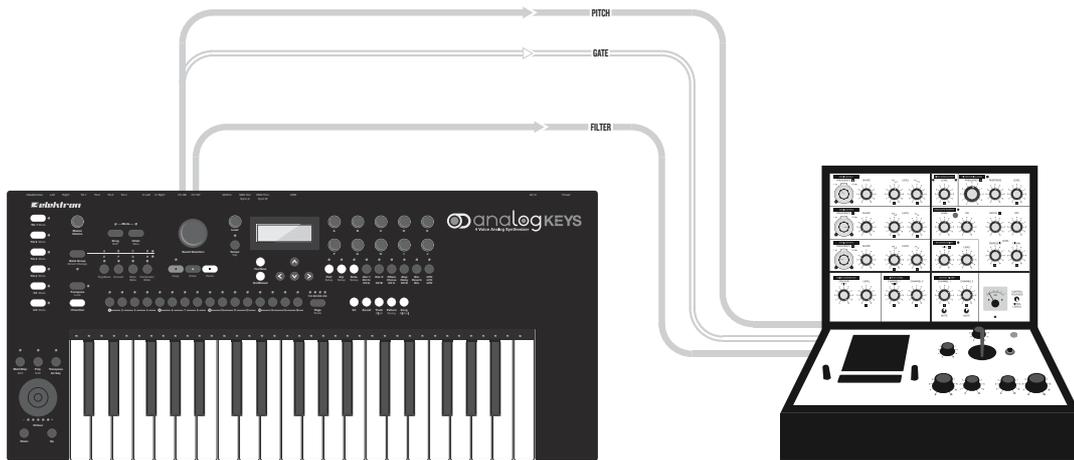
The CV/Gate track of Analog Keys is made for controlling external, CV/Gate equipped, analog gear. In this scenario, a vintage analog synthesizer is controlled by Analog Keys. The pitch and filter cutoff will be controlled.
