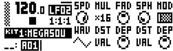
**SPD** (LFO2 Speed) sets the speed of LFO2. It is synced to the BPM. For LFO2 to be synced to straight beats, try settings of 16, 32 or 64. The value is bi-polar (the LFO shape can be played backwards by using negative values).
