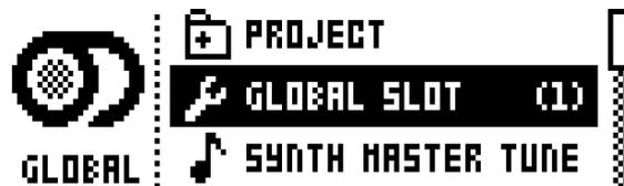
Scroll the list by using [UP]/[DOWN] or the LEVEL knob and select PROJECT. Open the menu by pressing [YES/SAVE].
