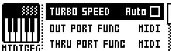
**TURBO SPEED** selects the multiplier of the MIDI transfer rate that will be used when the Analog Four MIDI IN/OUT ports are connected to the MIDI OUT/IN ports of a turbo protocol compatible device. The [LEFT]/[RIGHT] arrow keys are used to select the multiplier. If AUTO is chosen, press [YES/SAVE] to start the turbo speed negotiation.
