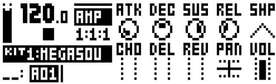
**ATK** (EnvA Attack) sets the attack time of the EnvA envelope, which controls the amplitude of the track.
