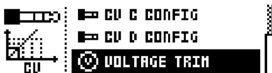
Make sure you have a good voltmeter before proceeding. Connect a TRS cable to the output you want to trim. Connect the volt meter's negative terminal to the sleeve of the connector. Connect the positive terminal to either the tip or the ring of the connector, depending on the channel you wish to trim.
