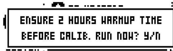
Press [YES/SAVE] to proceed with the calibration. Please note the calibration routine takes a while to complete.
