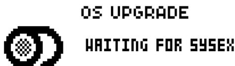
For the transfer to be possible, the device sending the OS syx-file should be connected to either the **MIDI IN** or **USB** port of the Analog Four. Cancel the waiting state by pressing **[NO/RELOAD]**.
