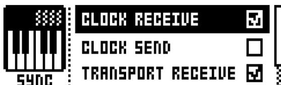
**CLOCK RECEIVE** will when active make the Analog Four respond to MIDI clock sent from external devices.
