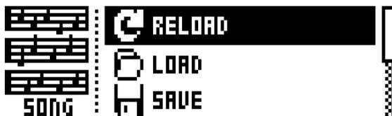
**RELOAD** will reload the active song. It will be restored to its saved version. Press [NO/RELOAD] + [KEYBOARD G1] for a short cut to this command.
