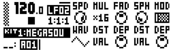
**SPD** (LFO2 Speed) sets the speed of LFO2. It is synced to the BPM. For LFO2 to be synced to straight beats, try settings of 16, 32 or 64. The value is bi-polar (the LFO shape can be played backward by using negative values).
