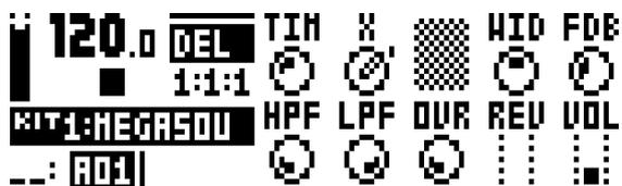
**TIM** (Time) sets the delay time. It is relative to the current BPM and is measured in 128th notes. For instance, a setting of 32 equals a one beat delay (four 1/16th notes).
