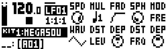
**SPD** (LFO1 Speed) sets the speed of LFO1. It is synced to the BPM. For LFO1 to be synced to straight beats, try settings of 16, 32 or 64. The value is bi-polar (the LFO shape can be played backward by using negative values).
