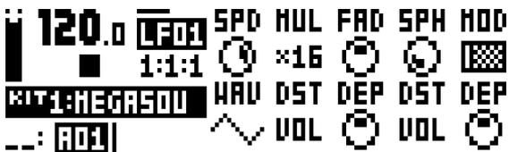
**SPD** (LFO1 Speed) sets the speed of LFO1. It is synced to the BPM. For LFO1 to be synced to straight beats, try settings of 16, 32 or 64. The value is bi-polar, meaning the LFO shape can be played backward by using negative values.
