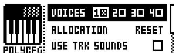
**VOICES** Select any combination of the four voices to be poly activated by using the [LEFT] and [RIGHT] arrow keys. Tick or untick a box by pressing the [YES/SAVE] button. To activate/deactivate voice 1-4 directly, press [TRIG] key 1 through 4. When in the POLY CONFIG menu, the red LEDs above [TRIG] key
