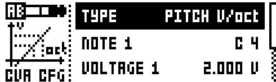
5. Set the SRC parameter of the CV A page to TR1. This will make the CV track send out pitch voltages according to the note trigs on synth track 1.
