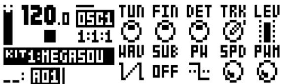
**TUN** (OSC1 Coarse Tune) sets the pitch of the oscillator in semi-tones. To jump a whole octave, press the knob while turning it.
