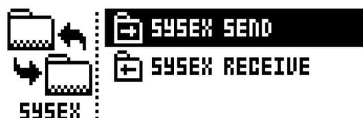
When receiving or sending SysEx data, the MIDI ports or the USB port of the Analog Four should be connected to the external sending/receiving device.
