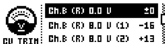
Each CV output has three trim settings. Begin by selecting 0 V, then press and hold the [YES/SAVE] key. 0 V is output as long as [YES/SAVE] is held down. Use [ARROW] keys [LEFT]/[RIGHT] or *DATA ENTRY KNOB A* to adjust the voltage until your voltmeter shows exactly 0 V. Repeat the process for both 8 V settings (the first one is for continuous voltage, the second is for pulse).
