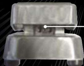
ADJUSTABLE ROCKER TORQUE: TURN THE ALLEN SCREW COUNTER-CLOCKWISE TO LOOSEN THE PEDAL; CLOCKWISE TO TIGHTEN (WRENCH INCLUDED)
