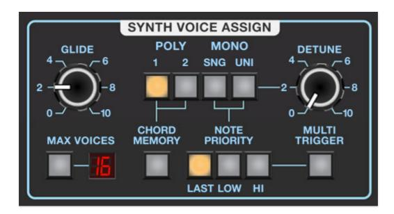
The Synth Voice Assign section determines how notes are assigned to the synthesizer section, i.e. Oscillators 1, 2, and 3. Controls in the Synth Voice Assign have no effect on the Strings section.
