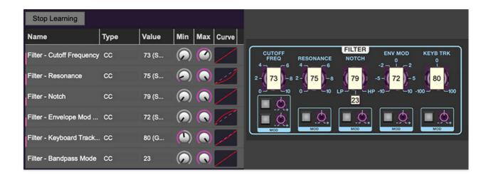
When in MIDI learn mode, any previously assigned controller numbers will show in squares. These indicate the MIDI continuous controller number of the assigned hardware control (these are also displayed in the *MIDI* library tab at left).
