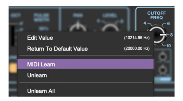
Begin by right-clicking on the *Cutoff Freq* knob in the Filter section and selecting *MIDI Learn*. A transparent purple overlay appears over the knob indicating that it's in learn mode. Now move the desired hardware control device. The purple overlay disappears and the hardware control will move the onscreen knob. If you get cold feet (or accidentally put the wrong control
