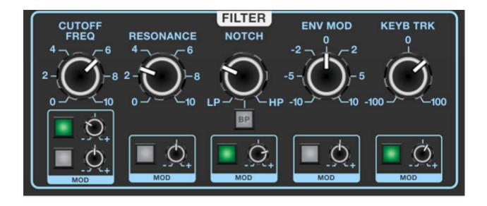
**Frequency**- Sets the frequency where frequency attenuation begins. Its effect dependent upon the currently chosen filter mode (lowpass, highpass, bandpass, or notch).
