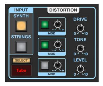
Dreamsynth's distortion effect operates in dual-mono mode; that is, it doesn't stereo-ize incoming mono signals, but incoming stereo imaging (i.e. panning the Synth or Strings) is maintained - the stereo image isn't summed to mono.
