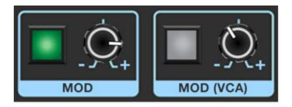
**Mod Source Select button**- Click to open a popup menu that selects the modulation source. If the button is dim (gray), no modulation source is currently selected. The button illuminates in green when a mod source is selected. (The attenuator still needs to be increased or decreased from its center position to apply mod.)
