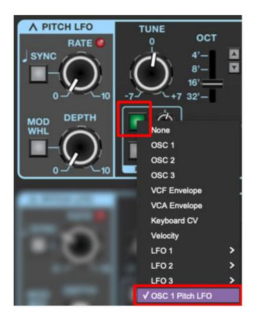
Set the Pitch LFO to the desired settings for one oscillator - in this example, we'll use Osc 1. Now we'll use Oscillator 1's Pitch LFO to modulate Oscillator 2.
