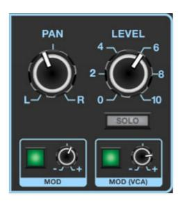
**Pan and Mod box** - Sets the oscillator panning position left to right. Remember that following the oscillators, Dreamsynth's audio path is fully stereo (including the filter section), so stereo pan positions are maintained. The *Mod* box beneath the *Pan* knob allows all manner of modulation of pan position.
