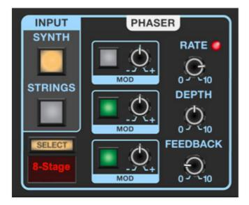
A super-sweepy phaser with multiple stage options. Generally speaking, the more stages a phaser has, the more "swooshy" the sound, but keep in mind that some of the world's greatest phasers used only four stages (MXR Phase 90 and Electro-Harmonix Small Stone come to mind).
