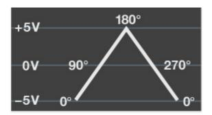
In the above diagram of a triangle wave LFO, the control voltage cycles from -5V through 0V, up to 5V, back down through 0V, down to -5V, etc. The phase setting corresponds to *where* in the waveform the control voltage is "tapped." If the LFO is being used for an application such as pitch mod (vibrato) or repeating filter wahwah, you won't hear any audible difference between phase settings. But here's an example of where multiple LFO phases can be useful:
