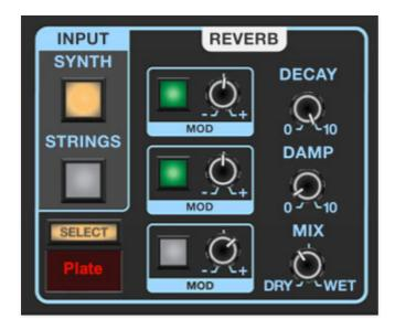
A smooth, studio-quality stereo reverb. The stereo implementation allows it to be used to stereoize mono (i.e. centered) sounds, but panning positions are retained.
