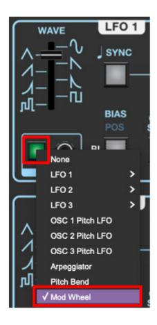
Another method to get equal pitch mod for all oscillators would be to assign one of the main LFO's to multiple oscillators' Pitch Mod sections. Mod wheel-controlled depth can be set up by clicking the LFO's mod source pop-up and selecting *Mod Wheel*, then turning up its associated attenuator.
