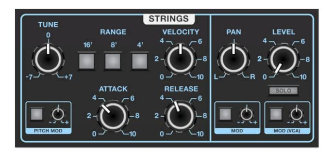
The Strings section emulates a classic, "top-octave divide" string synthesizer. Like vintage string synths, the signal is routed to an always-on "tri-chorus" - a clever and really great-sounding implementation of chorus seen in a number of 70s strings machines that used three BBD delay chips with six modulation sources to create that lovely, syrupy string chorus sound made famous by the Solina String Synthesizer.
