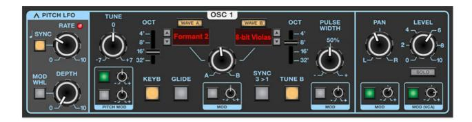
Dreamsynth's three dual-waveform oscillators are perhaps its most special component. The basic concept is that each oscillator simultaneously outputs two virtual analog or sampled waves, with their blend set either manually, or CV-controlled via one of Dreamsynth's numerous mod sources.
