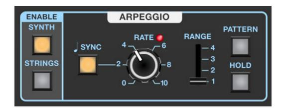
An arpeggiator is basically a step sequencer that plays each note of a chord individually in a pattern across one or more octaves.
