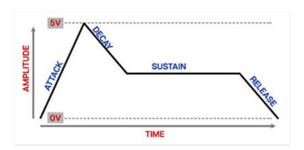
When Dreamsynth sees a gate voltage from a note, the envelope generator outputs a dynamically changing voltage, according to the settings of its four stages. The attack stage defines how long it takes for the output voltage to rise from 0 to 5 volts. Once the attack stage reaches 5V, it moves to the decay phase, which defines how long it takes to fall from 5V to the setting of
