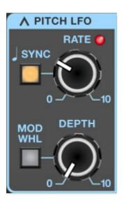
Each oscillator has its own dedicated triangle-wave low-frequency oscillator, hard-wired to oscillator frequency. These let you add oscillator vibrato without having to "waste" one of the main LFO's (which can be used for more serious sound mangling!). Note that **the Pitch LFO always affects wave A and B equally**.
