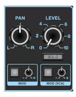
**Pan and Mod box** - Sets the Strings panning position left to right. The *Mod* box beneath the *Pan* knob allows modulation of pan position.
