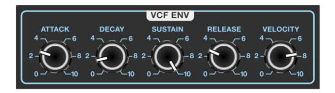
**Attack**- Defines the length of time for voltage to rise from 0V to 5V when a key is played.
