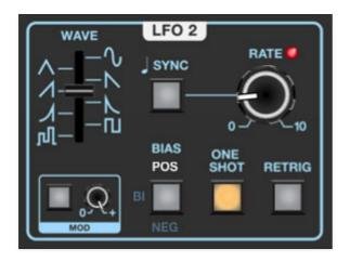
Set LFO 2 Wave to the ramp position, Bias to Positive, enable One Shot, and set Rate to around 1 Hz (when an LFO is in One Shot mode, the Rate knob defines the length of the single wave cycle.)
