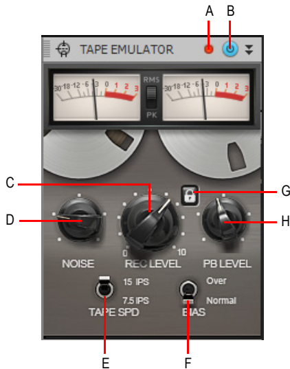
A. Clipping LED B. Tape Emulator enable/disable C. Rec level (input gain) D. Noise (tape hiss) E. Tape speed F. Bias G. Stereo link H. Playback level
