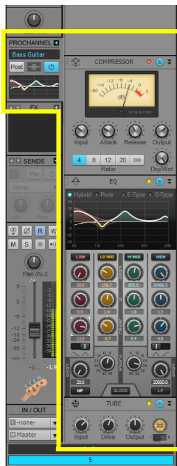
Figure 306. ProChannel provides compressor, equalizer and tube saturation processing for each channel.
