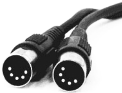
Figure 1. Standard MIDI cable—use this if your MIDI interface has standard 5-pin input and output ports
