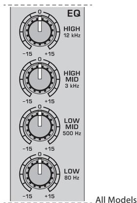
Fig. 2.2: Equalizer of the input channels
