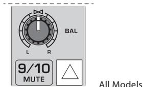
Fig. 2.6: Balance control and mute switch
