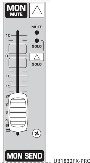
Fig. 2.11: Monitor fader of the UB1832FX-PRO
