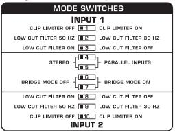
Fig. 2.3: DIP-switches
