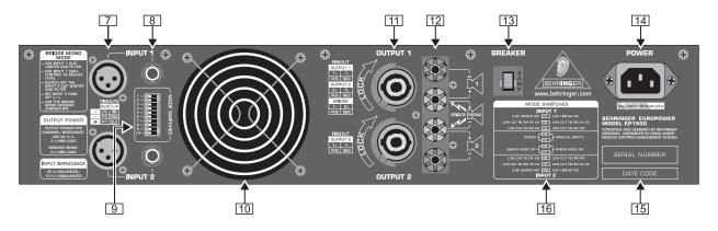
Fig. 2.2: Rear panel control elements
