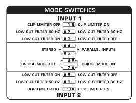
Fig. 3.6: DIP switch positions for mono-bridged mode
