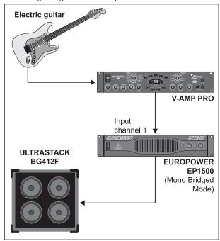
Fig. 3.5: Mono-bridged mode
