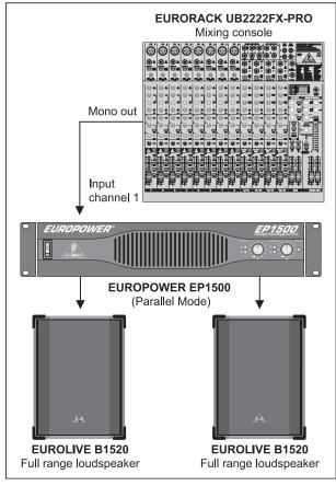
Fig. 3.3: Parallel operation
