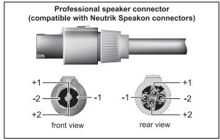
Fig. 4.1: Neutrik Speakon-compatible connectors
