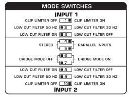
Fig. 3.4: DIP switch positions for parallel operation
