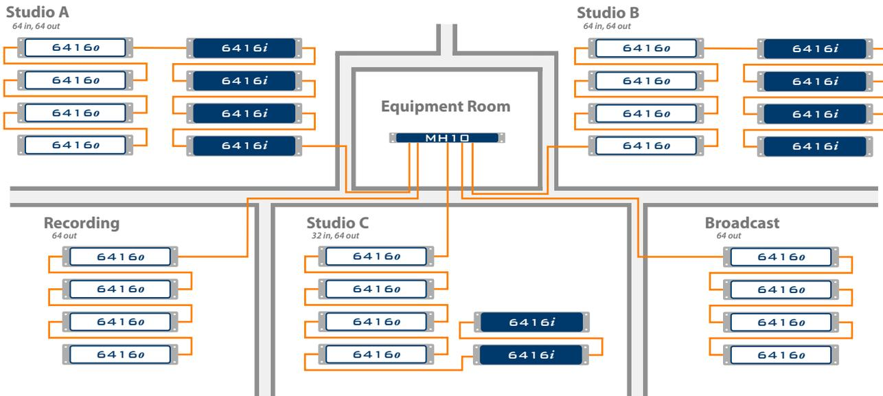
**Everything Everywhere.** Up to 64 channels, from any combination of the three studios, can be inserted into the network. All channels are available for output at every location shown here. Network topology has no impact on availability of channels; modules can be connected in the most convenient manner.
