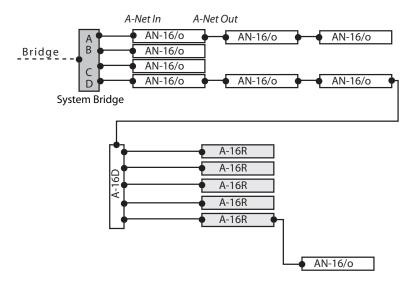
Port A of the System Bridge has a serial split with three output modules; port D splits serially to output modules and then in parallel to Personal Mixers and then serially again to another output module.
