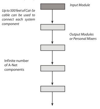
The distance between each A-Net device can be up to 500 feet (150 meters).
