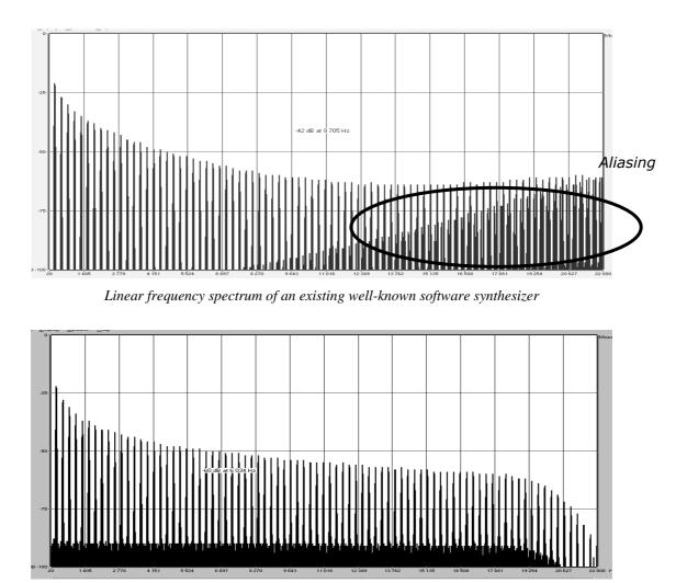
Linear frequency spectrum of the Moog Modular V oscillator made with TAE®
