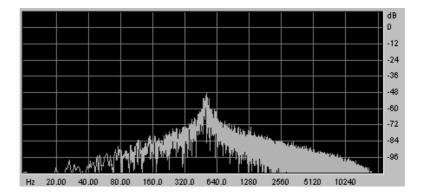
The band-reject (band-reject filter or notch) eliminates the frequencies inside a band of frequencies. This filter is above all else interesting when we want to vary this band of frequencies (with the "frequency" on the Moog Modular V filters or the modulation of an LFO on this same parameter). You will thus obtain a sound close to a "phasing" effect.
