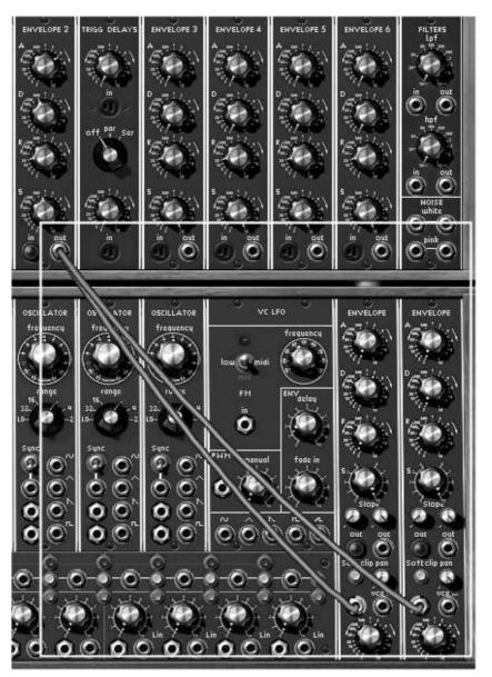
Connection of an auxiliary envelope for the output VCA
