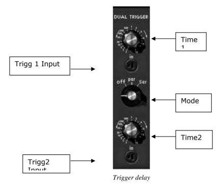
Time 1: Sets the time for the first delayTrigg 1 Input: Choice of trigger input for the first delayMode: Choice of mode (independent, parallel, series)Time 2: Sets the time for the second delayTrigg 2 Input: Choice of trigger input for the second delay
