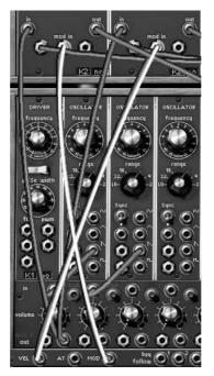
Connections for modulation and velocity outputs on the frequency modulation of filters 1 and 2
