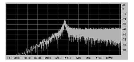
The band-pass (band-pass filter or BPF) eliminates the frequencies situated on either side of the cut-off frequency. Use it to make a certain band of frequencies that you wish to emphasize appear. This will make the sound more "pinched".
