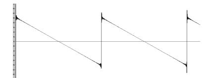
Temporal representation of the waveform of an existing Moog-like software synthesizer
