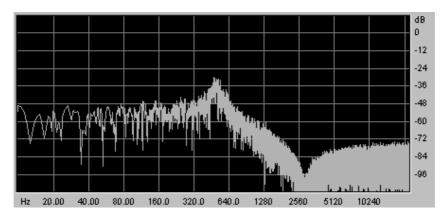
The high-shell filter increases or decreases the frequencies above the cut-off frequency (with the action of the gain knob).
