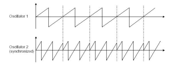
In the image above, oscillator2 is synchronized with the first, and then tuned to a frequency with double the tonality.
