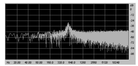
The bell filter amplifies or dampens a frequency band (in function with the gain knob)
