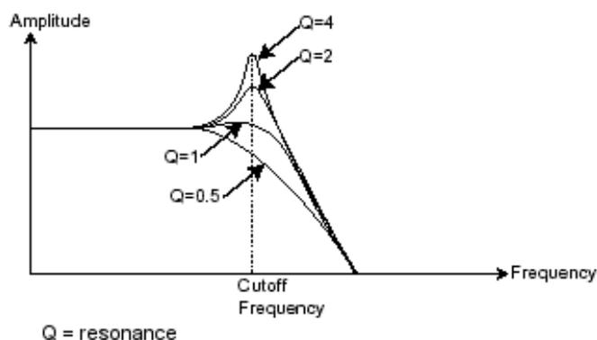
With a high resonance level, the filter will begin to produce a sound close to a sine waveform. At this stage, the use of a key follow is very important as you can create a melody by tuning the cut-off frequency of the filter along with the frequency of the oscillators.
