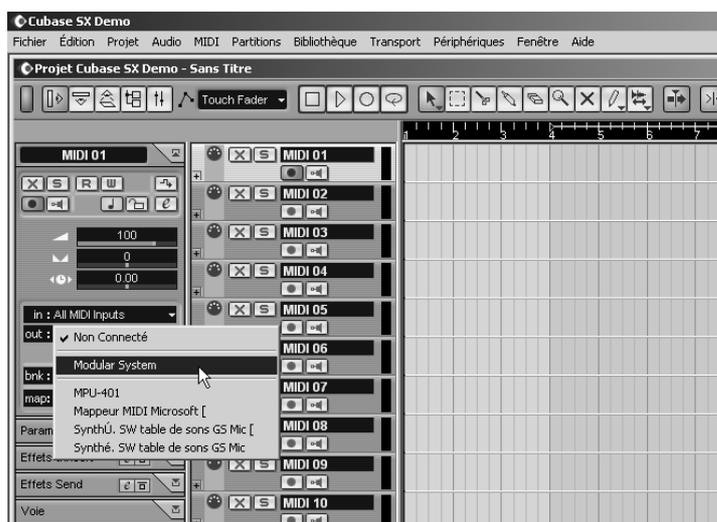
Connection of a MIDI track to the ARP2600 V
