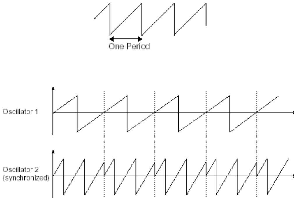
*In the above image, oscillator2 is synchronized with the first and tuned to twice its frequency. The resulting waveform is unique in that it cannot be created by standard synthesis techniques such as layering or filtering.*
