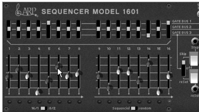
*The two lines of faders and selector switches*
