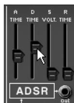
*The “Decay time” parameter on the filter envelope*
