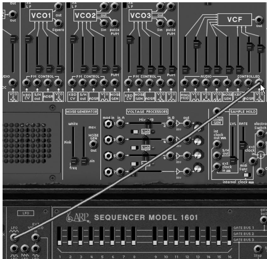
*Modulate the filter frequency (“Cutoff Frequency”) with the LFO*
