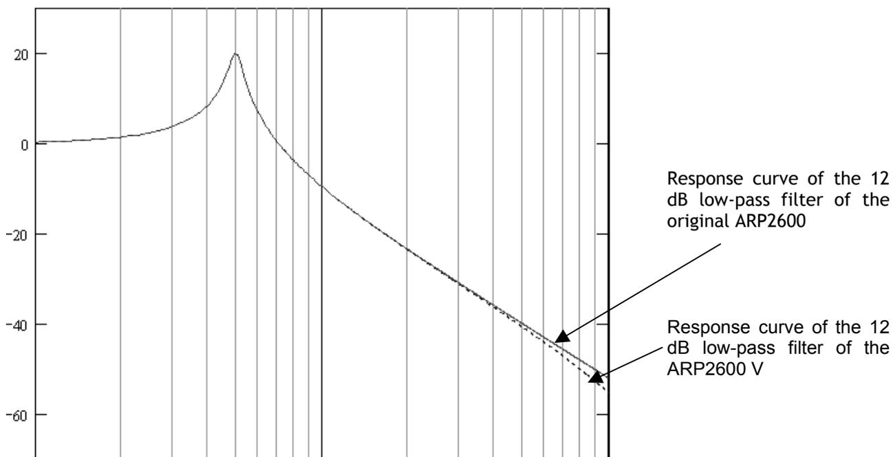
*Response curve of the 12 dB low-pass filter of the original ARP2600 V and the ARP2600 V*
