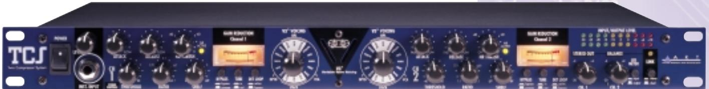
The TCS is a two-channel high performance compression system which features two types of compression per channel utilizing ART's Dual Topology technology.
