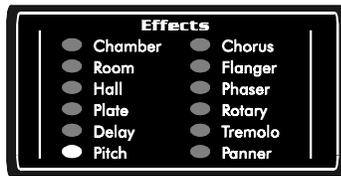
The Pitch Transposer (PT) algorithm can change the base-pitch of a sound. Each PT class contains an auxiliary digital delay that feeds back into the pitch shift. This feature can create falling or rising pitch effects. Some classes also have dynamics sensing, which can use input level to switch the effect in and out or trigger the *Whammit!* effect (see *Dynamic* class).
