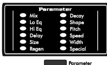
If you wish to change the value of any of the effect's parameters, press the Parameter button and use the Encoder to scroll through your choices. All available parameter LEDs remain lit, but now the currently selected parameter is flashing and its value is shown in the Preset / Value Display. When you have chosen the parameter that you want to edit, press the
