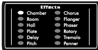
The Chamber Reverb simulates a reflective enclosure (perhaps made of wood or concrete) with a sound source at one end and a microphone near the other. By varying the Size parameter from small to large, you can simulate spaces as small as a shower stall and as large as an elevator shaft. This reverb is more reflective and has a more defined echo characteristic than Halls or Rooms.
