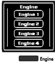
The Quadra/FX contains up to four audio signal processors, or engines. Pressing this button and turning the Encoder will select an engine for editing (the selected engine LED will flash). Depending on the current routing, one or more engine LEDs may flash. Press the Engine button again to return to Preset mode. For more information on engines, see page 27.
