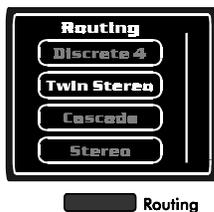
By editing any preset's routing, you are essentially building a new preset from scratch. When routings are changed, the Quadra/FX reconfigures its internal architecture and loads in default effects. The preset's former effects, class, and parameter values are all replaced.
