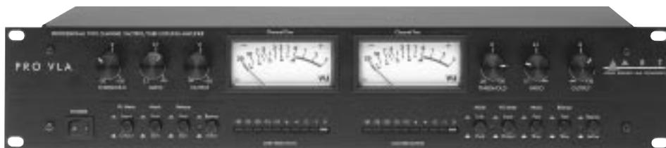
The PRO VLA (Vactrol-based Leveling Amplifier) is a multi-purpose tool for audio engineering and recording. Its two independent (and stereo link-able) channels of analog leveling/compression are designed to work seamlessly with any recording, sound-reinforcement, or electronic instrument setup. A VCA-less design utilizes optical electronics (Vactrol) coupled with a 12AX7 vacuum tube gain stage for superior musical performance.
