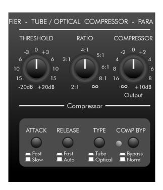
array). Now adjust Threshold (either lower or higher) until you have the desired amount of compression. (Use the Gain Reduction LEDs as a visual guide)
