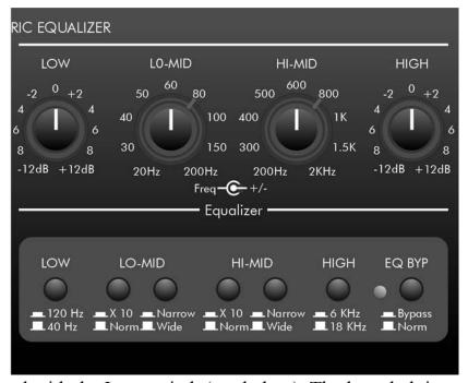
The two frequencies are selected with the Low switch (see below). The low shelving filter affects all frequencies below the corner frequency when applying boost or cut. In other words, cutting at 40Hz also cuts 30Hz, 20Hz, etc. The Low control has as range of  $\pm 12$ dB.
