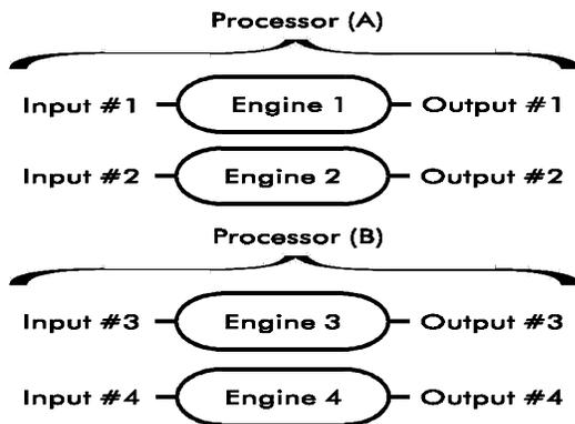
In Discrete 4 routing, each engine separately processes one channel of sound and is just like having four mono effects. Inputs and Outputs #1–4 correspond to Engines #1–4. Engines #1 and #2 are edited in Processor (A) and Engines #3 and #4 are edited in Processor (B).
