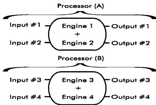
This routing turns the DMV-PRO into two true-stereo processors. Inputs #1 and #2 feed the first processor (consisting of grouped Engines #1 and #2) and exit at Outputs #1 and #2, and Inputs #3 and #4 feed the second processor (consisting of grouped Engines #3 and #4) and exit at Outputs #3 and #4. The left and right audio channels of each processor remain separate, but any modulated parameter, such as the LFO Speed for a chorus, is linked for both channels. With reverbs,
