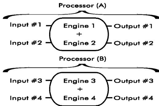
Twin Stereo routing contains two effect-processors with two linked engines each. The result is two true-stereo effects. Each channel's audio remains independent, but the effect parameters of each group are linked to create stereo processing. The first effect (Inputs, Outputs, and Engines #1 and #2) is edited in Processor (A) and the second effect (Inputs, Outputs, and Engines #3 and #4) is edited in Processor (B).
