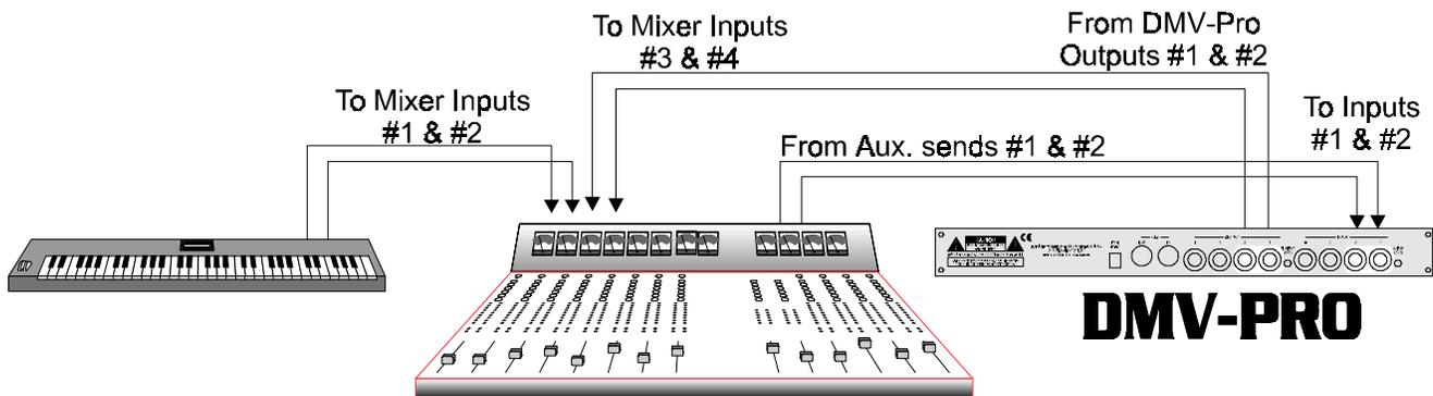
Connect two cords with ¼" plugs between your mixer's auxiliary sends and the DMV-PRO's Inputs #1 and #2. For a mixer with a mono send, use only Input #1. Connect Outputs #1 and #2 to two input channels or the returns on your mixer.
