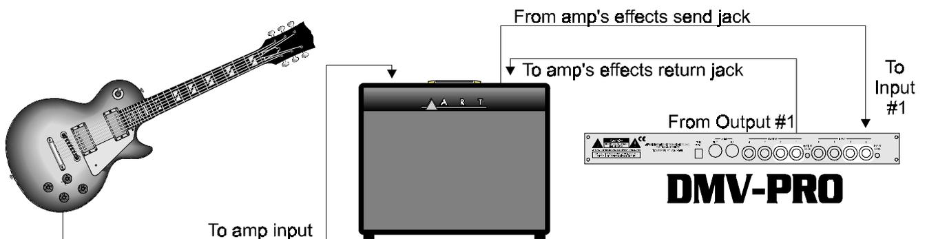
If you're patching the DMV-PRO into a guitar (or other instrument) amplifier's mono effects loop, use one cord between the amp's Effects Send jack and the DMV-PRO's Input #1. Run a second cord from Output #1 to the amp's Effects Return jack. (If the amp has stereo returns, use another cord to connect the DMV-PRO's Output #2 to the amp's other Effects Return jack.) Again, don't forget that the DMV-PRO has the power to act as two separate, stereo processors or four separate, mono processors.
