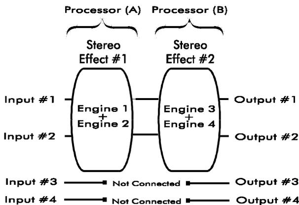
This routing feeds the output of one stereo processor (grouped Engines #1 and #2) into another (grouped Engines #3 and #4). It only uses Inputs and Outputs #1 and #2; Inputs and Outputs #3 and #4 are disabled. As with Twin Stereo, the left and right audio channels of each processor remain separate, but modulated parameters are linked.
