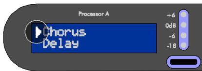
The Selection Arrow appears on the left side of an LCD and is used to distinguish the active line. For example, in the picture on the right, the Selection Arrow indicates that Chorus is the selected effect and it will be affected by turning the encoder or pressing the Edit button. To select the other line, press the same processor's encoder. While editing, the Selection Arrow is used to differentiate the active parameter or value field.
