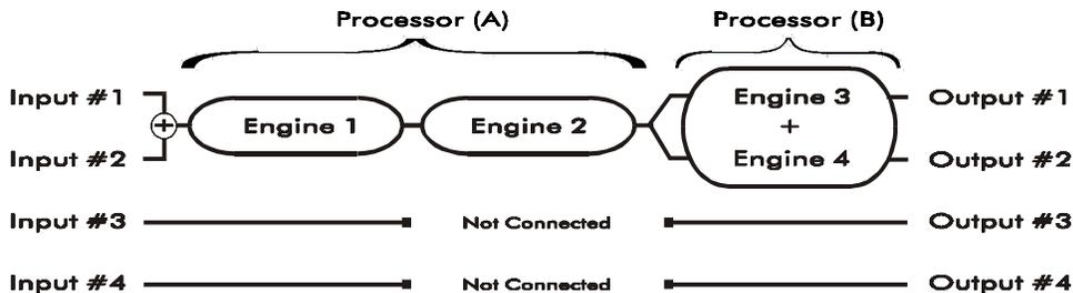
Multi FX routing uses the DMV-PRO's processors to create a three-engine multi-effect chain. Since most engines contain a separate effect, EQ, delay, and dynamics sensing section, the actual multi-effect lengths can be quite long. This routing gives you tons of power to creatively shape your sound.
