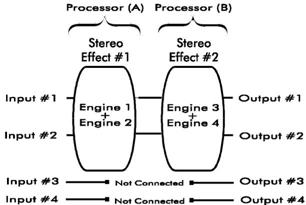
Cascade routing also has two effects with two linked engines, but the output of the first group is fed into the second. In this routing, you have two stacked, true-stereo effects. Only Inputs and Outputs #1 and #2 are used. The first effect (Engines #1 and #2) is edited in Processor (A), and the second effect (Engines #3 and #4) is edited in Processor (B).
