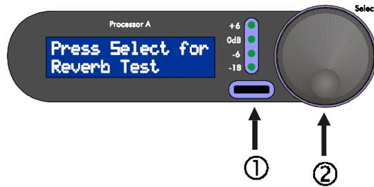
Smart Encoder functions are automatically set up to work while editing reverb, delay, and rotary effects. For *Reverb* effects, a reverb impulse can be triggered while adjusting any of the reverb's parameters; this helps you hear the reverb changes as you are making them. To trigger an impulse while editing, simply press and hold the Edit button of the corresponding processor and press the Encoder. As soon as the Encoder is pressed, the impulse will fire. Repeat as often as necessary.
