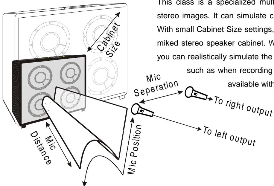
This class is a specialized multi-tap delay system for creating stereo images. It can simulate close and far miking techniques. With small Cabinet Size settings, this algorithm emulates a close miked stereo speaker cabinet. With large Cabinet Size settings, you can realistically simulate the miking of a wide speaker array, such as when recording a live concert. This class is not available with a mono routing.
