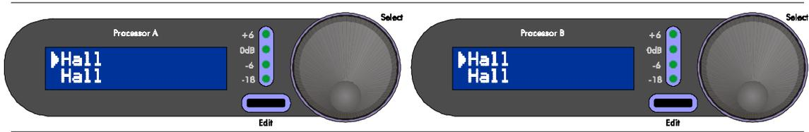
Look at LCD (A). The top line now corresponds to Effect #1 (at Input and Output #1) and the bottom line corresponds to Effect #2 (at Input and Output #2). Processor (B) is similar, with its top line representing Effect #3 and its bottom line representing Effect #4. Notice the “Selection Arrows” on the top-left of both lines. These arrows indicate that the top effect is the one that will change when the corresponding encoder is turned.
