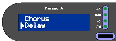
The DMV-PRO contains two Liquid Crystal Displays—LCD (A) and LCD (B). Both displays separately show information about their corresponding processor and when the MIDI/Util button is pressed, they both work together for viewing global parameters.
