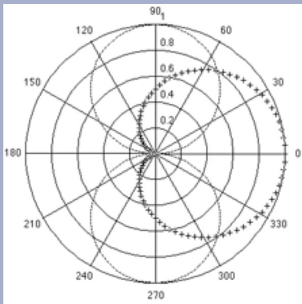
*Directivity patterns for a bi-directional (--) and cardioid (++) microphone in M-S recording configuration. This reflects the physical configuration of the microphones in the original recording session.*
