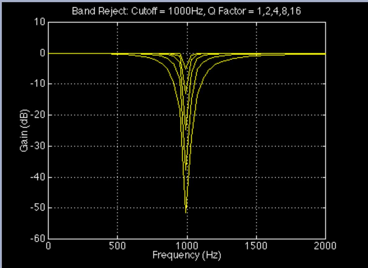
*Approximate response curves for the Band Reject filter at a fixed center frequency, but at various  $Q$  values. At a  $Q$  of 1, the dip in the center is smooth.*
