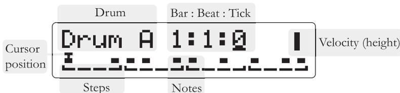
In the top line, the screen indicates that *Drum A* is being edited in *Step* mode.
