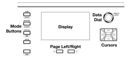
Advance 49's display shows information about its current mode and operations. You can navigate its different modes, pages, etc. by using the following controls:
