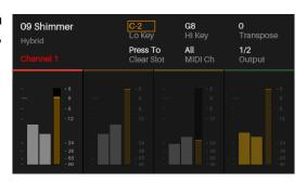
You can also add patches to a channel while in Multi Edit Mode. Press the **Browse** button to open the Browser and use the **Data Dial** and **Cursors** as you would in Browser Mode (described in **Browser Mode** > **Loading Patches**) to select and load a patch. That patch will then be loaded to the channel of the multi.
